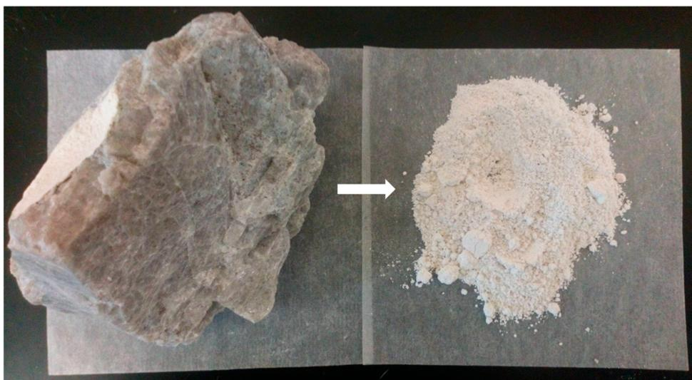
**Figure 1.** Imergard™WP before and after processing. Perlite, the active ingredient of Imergard™WP, is a volcanic rock (**left**) that can be expanded (when heated to 760–980 °C) and then processed (drying and grinding) to obtain the fine white powder used in this study (**right**).
