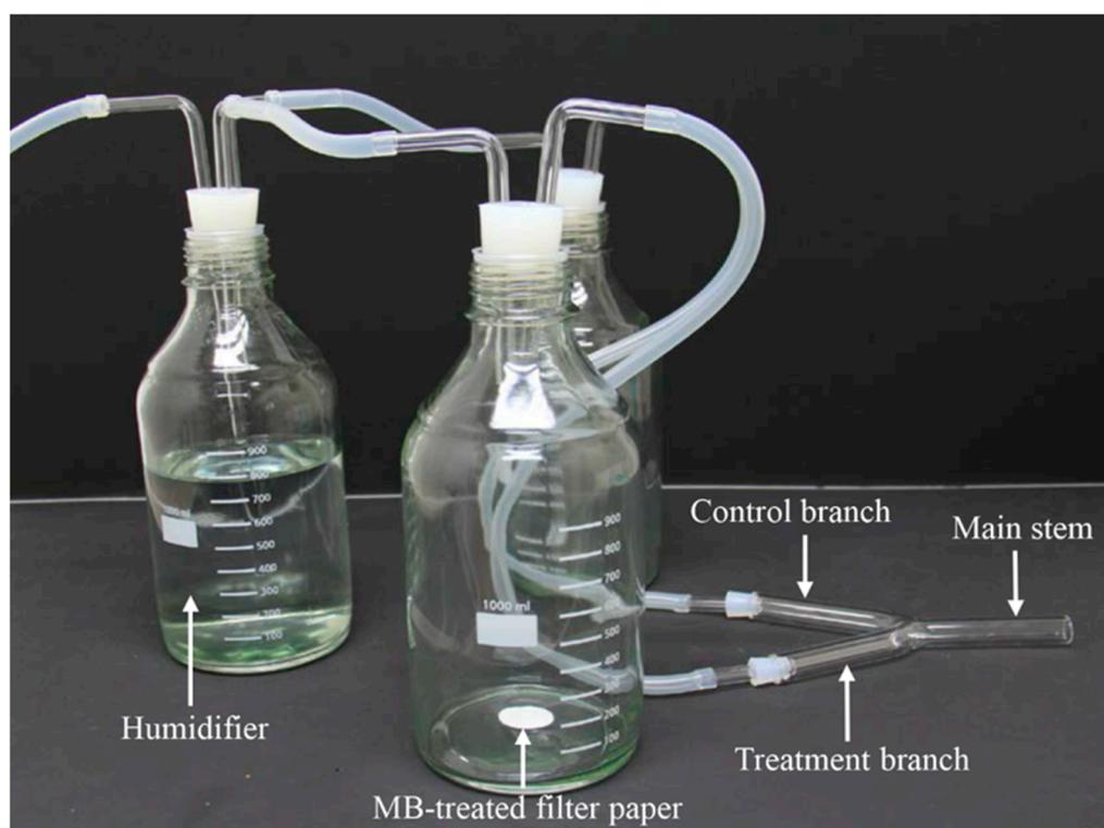
**Figure 1.** Y-tube olfactometer apparatus used to investigate the olfactory responses of adults of *Nesidiocoris tenuis* to methyl benzoate (MB).
