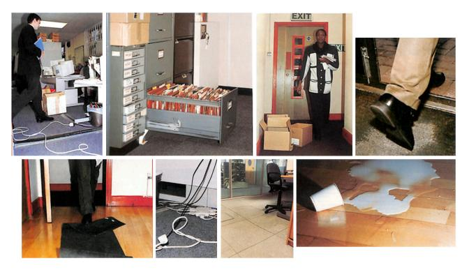
Figure 2. Potential 'slip, trip and fall' hazards. British Safety Council Archive.
