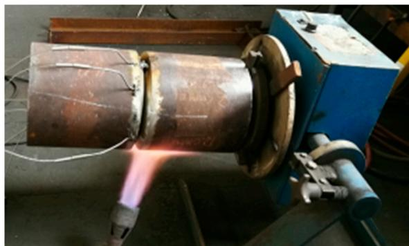
Figure 2. Pre-heat treatment of 12Cr1MoV pipe welded joint.
