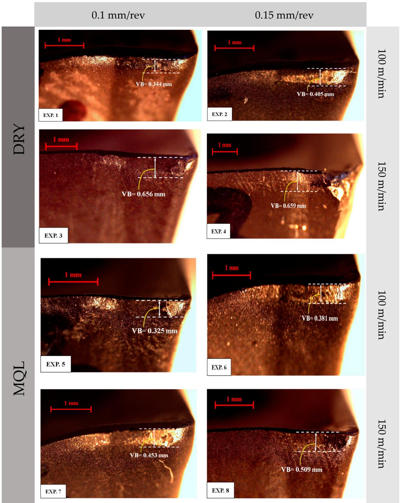
**Figure 2.** Progressive tool wear for each experiment provided as 0.344 mm, 0.405 mm, 0.656 mm, 0.659 mm, 0.325 mm, 0.381 mm, 0.453 mm, 0.509 mm from 1st to 8th experiments.
