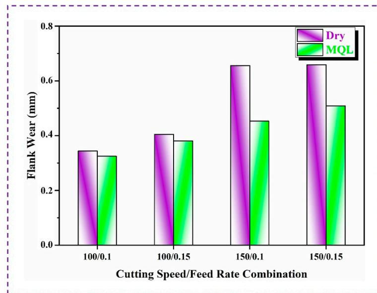
Figure 3. Effects of the cutting environment on the flank wear.
