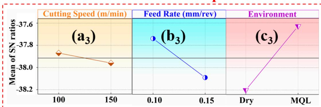
**Figure 6.** Signal-to-noise ratios for the (a1–a3) tool wear, (b1–b3) cutting temperature, and (c1–c3) power consumption related to the tool wear, cutting temperature, and power consumption.
