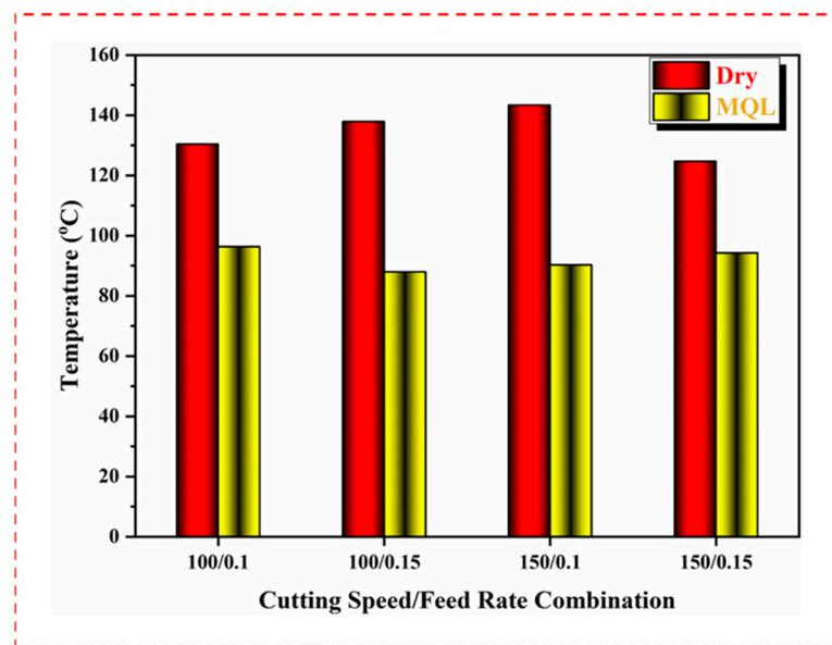
**Figure 4.** Effects of the cutting environment on the cutting temperature.
