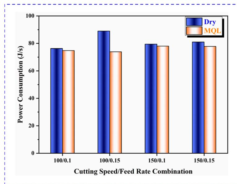
Figure 5. Effects of cutting environment on power consumption.
