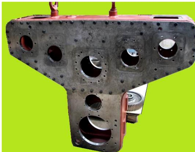
**Figure 3.** Adder box housing before mounting the covers and gears.
