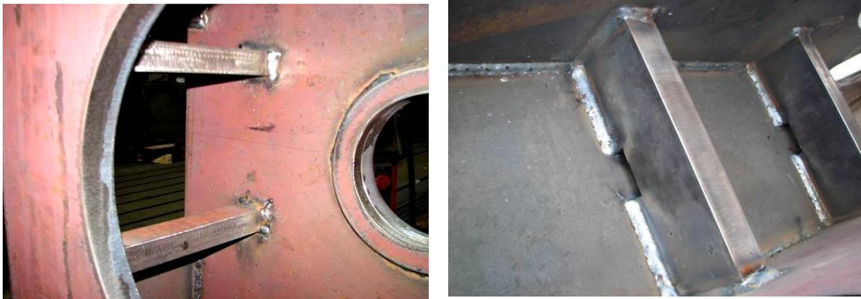
**Figure 18.** New adder box with reinforcements.
