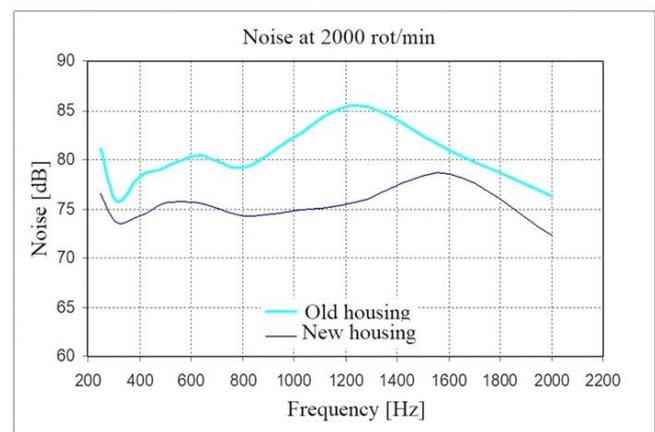
Figure 35. Lp sound pressure level diagrams for left side surface at 1500 and 2000 rpm.
