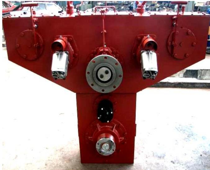
**Figure 17.** New adder box, welded version.
