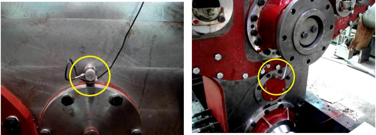
**Figure 19.** Acceleration transducer mounted at point No. 2 and 3 measures. Accelerometers are highlight with a yellow circle.
