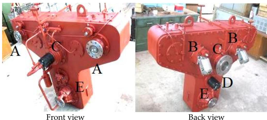
**Figure 2.** Adding box CSD 4000. (A) The input shafts; (B) Intermediate shafts I; (C) The shaft of the power take-off; (D) Intermediate shaft II; (E) The output shaft.
