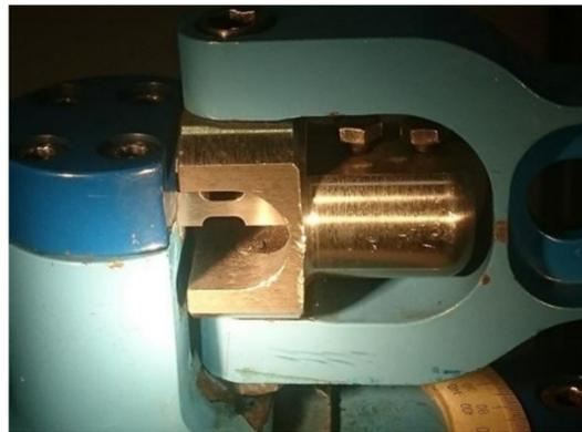
**Figure 3.** Clamped specimen in MZGS-100 machine.
