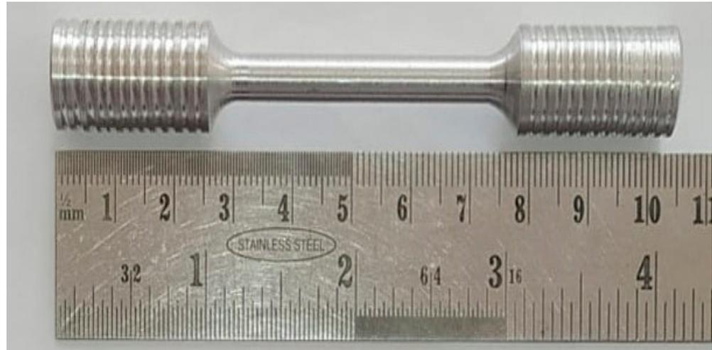
**Figure 1.** Tensile test specimen as per ASTM D3552-17.
