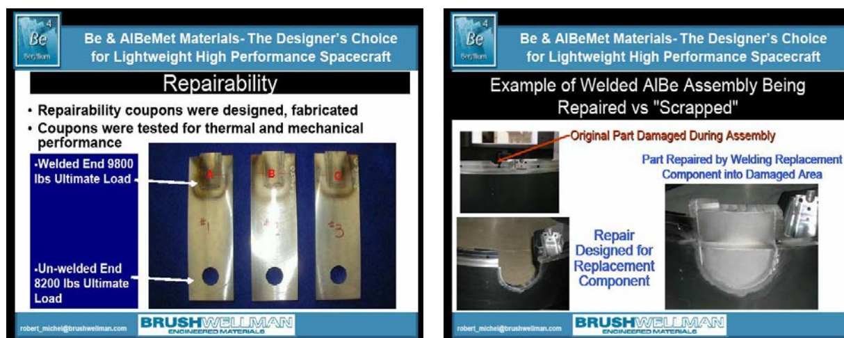
Figure 11. The EBW repaired sections of Be-Al alloy [62] Reprinted/adapted with permission from Ref. [62] Copyright 2008, SPIE.
