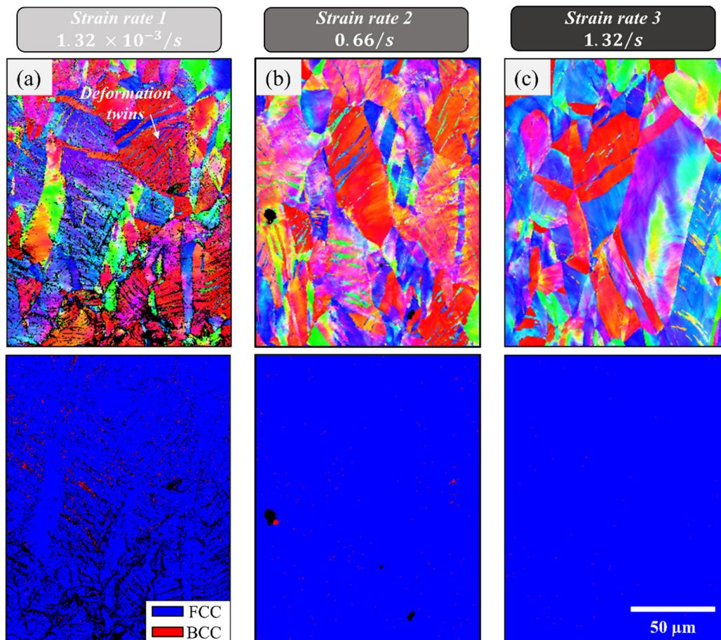
**Figure 7.** (a) EBSD grain orientation and phase maps of a sample deformed at RT and  $1.32 \times 10^{-3}/s$  deformation rate. (b) RT and 0.66/s deformation rate. (c) RT and 1.32/s deformation rate.
