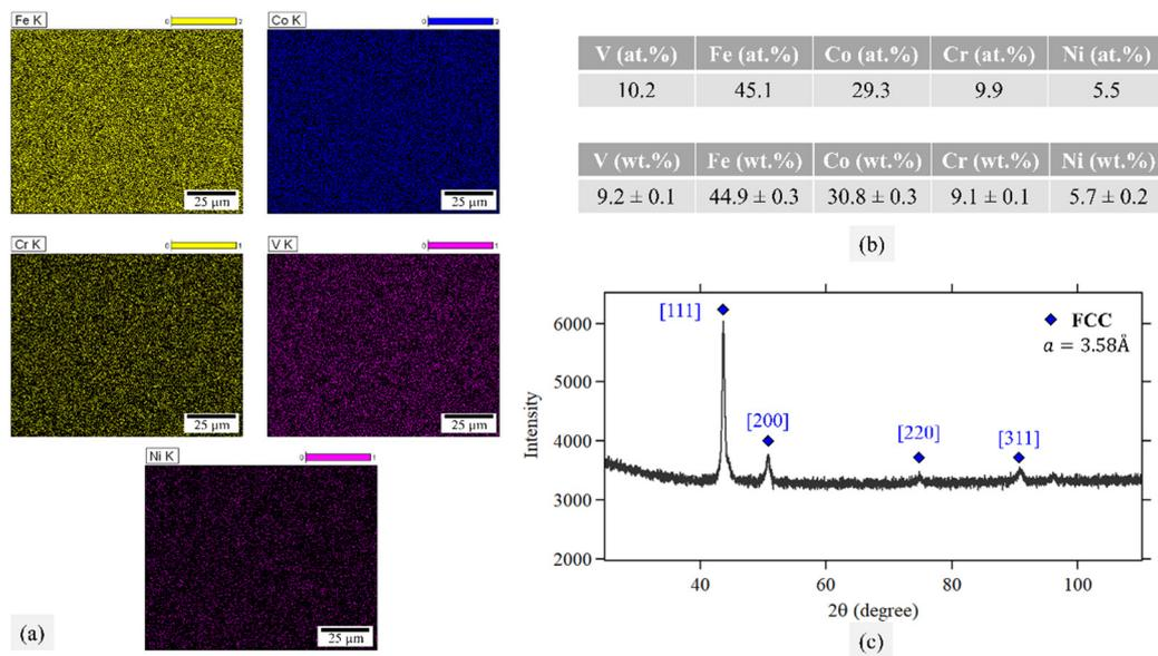
**Figure 1.** (a) EDX maps of Fe, Co, Cr, V, and Ni confirming the ingot's homogeneity. (b) The nominal composition in wt.% and at.%. (c) XRD analysis of a specimen following homogenization and solution heat treatments. The results point to a single FCC phase with a lattice parameter  $a = 3.58 \text{ \AA}$ .
