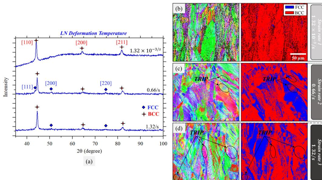
**Figure 11.** (a) XRD analysis collected from fractured samples deformed at  $-196$  °C and the three considered deformation rates. (b) EBSD grain orientation and phase maps of a sample deformed at  $-196$  °C and  $1.32 \times 10^{-3}/s$  deformation rate. (c)  $-196$  °C and 0.66/s deformation rate. (d)  $-196$  °C and 1.32/s deformation rate.
