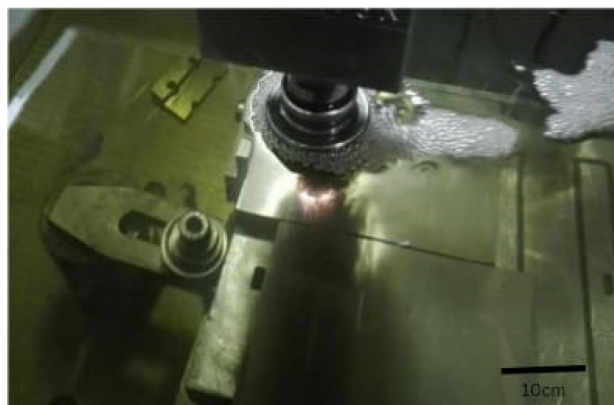
Figure 3. The phenomenon of spark erosion in AISI D2 Steel.
