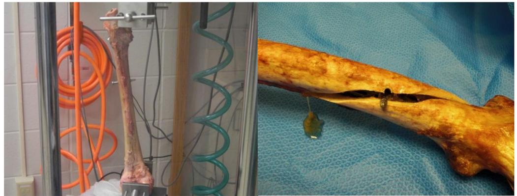
**Figure 6.** The femoral bone with the nail testing setup in the EnduraTEC BOSE machine (**left**). Model failure due to torsion (**right**). Reprinted from Ref. [31].
