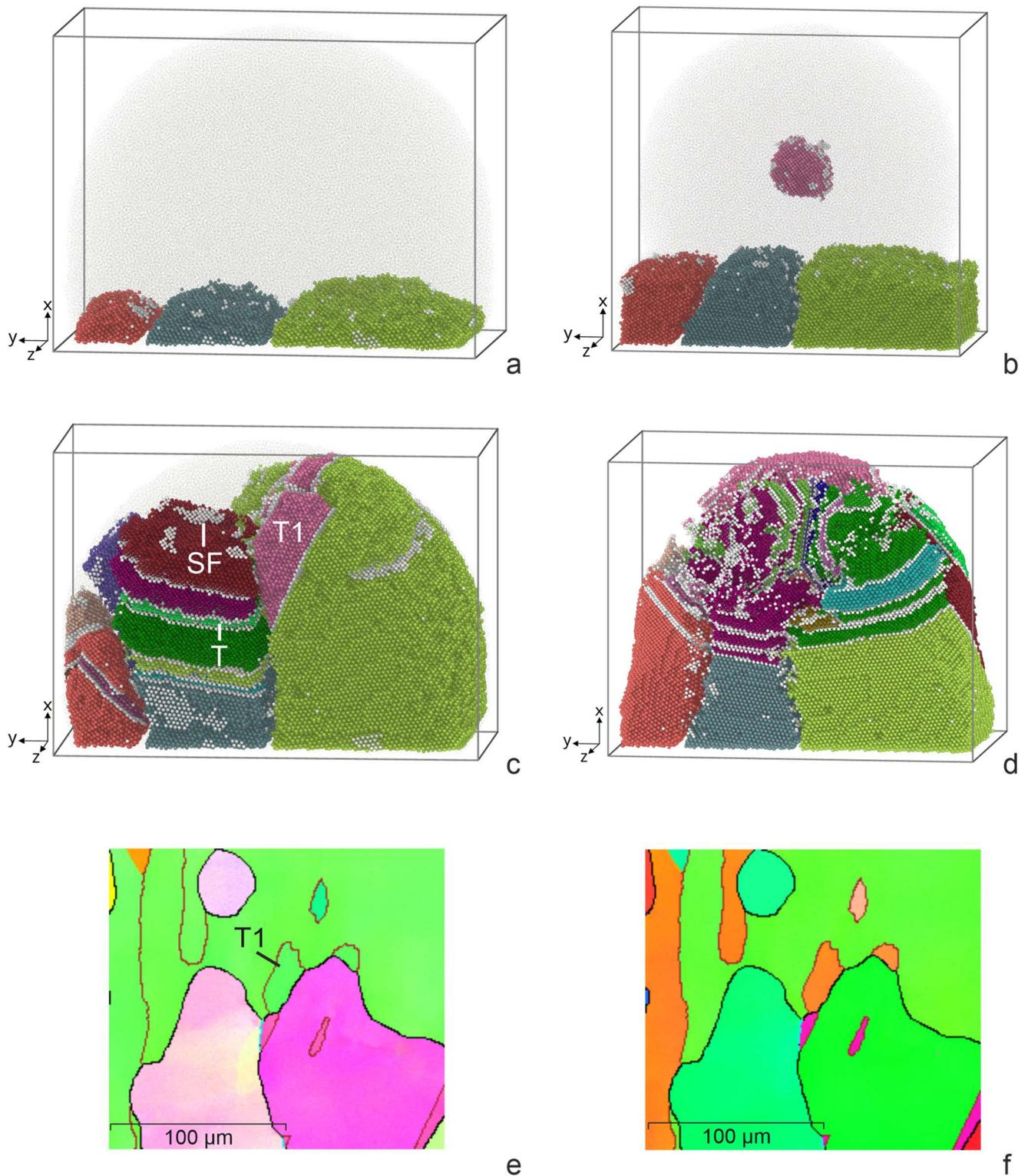
**Figure 7.** The structural changes during the interaction of a drop of melted aluminum bronze with the crystallized base (a,b) and subsequent crystallization (c,d) compared to orientation maps relative to the X (e) and Y (f) axes.
