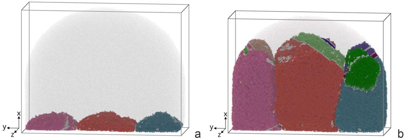
**Figure 10.** The melting of the deformed base (a) with the melting drop with a temperature of 2000 and subsequent crystallization of the drop (b).
