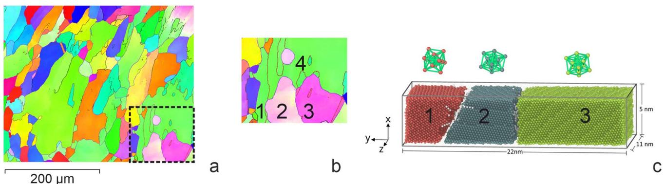
**Figure 5.** Area selected for simulation (b) on the orientation map (a) (section b in Figure 2) and the structure of the model before interaction (c) (1–4 are grains whose parameters were put into the model). Here and below, the colors show the atoms belonging, according to PTM, to different grains. Small dots show atoms that do not have a definite crystal structure (melt, interfaces, structural faults, etc.). Atoms located at the sites of the HCP lattice are marked in white.
