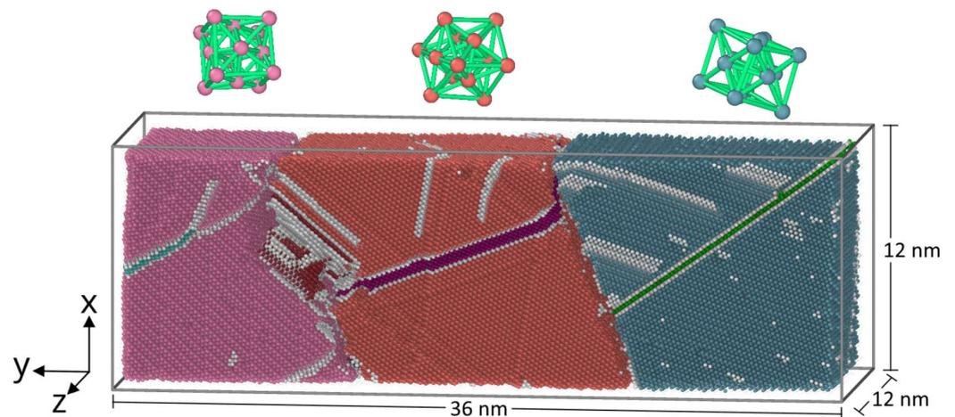
**Figure 6.** Three-grain model structure after deformation before interaction with a melt drop.
