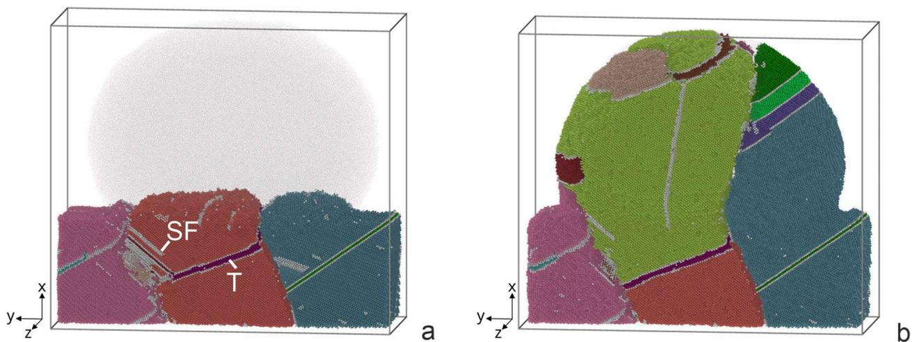
**Figure 8.** The structural changes during the interaction of a drop of melted aluminum bronze with the deformed base (a) and subsequent crystallization (b) (the drop temperature being 1380 K).
