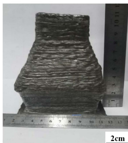
Figure 16. The final form of the thin-walled parts in the DED-Arc control process.
