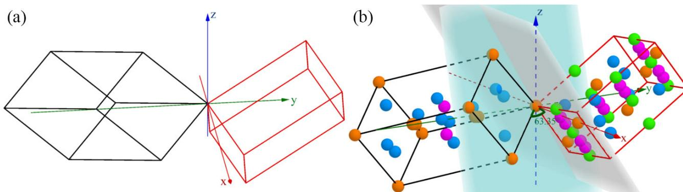
**Figure 8.** Oriented structural models described with cell edges (a) and unit cell (b) for  $\text{Al}_{12.48}\text{Fe}_{6.52}$  and  $\text{Al}_{5.72}\text{Fe}_2$  phases.
