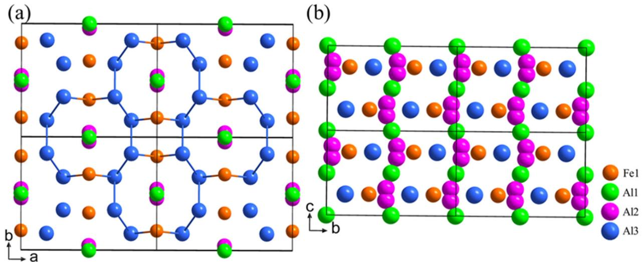
**Figure 6.** Projection of the  $Al_{5.72}Fe_2$  supercell along directions: (a) [001] and (b) [100].
