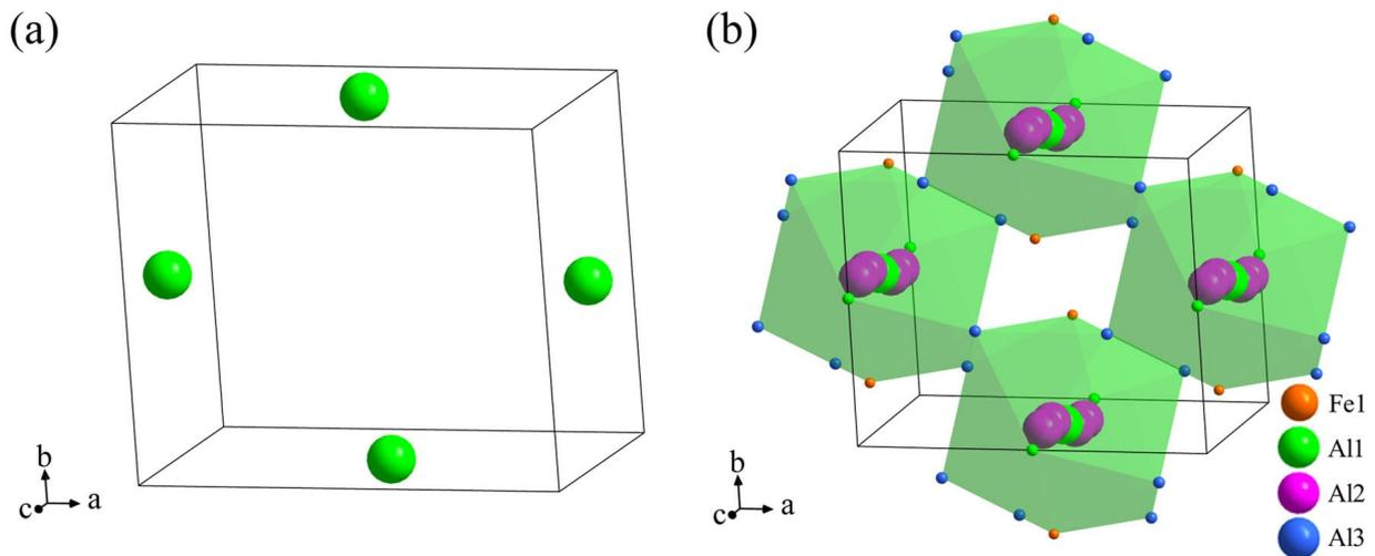
**Figure 7.** Cluster assembly in  $Al_{5.72}Fe_2$  phase cell: (a) The central atom of the cluster; (b) Cluster assembly model.
