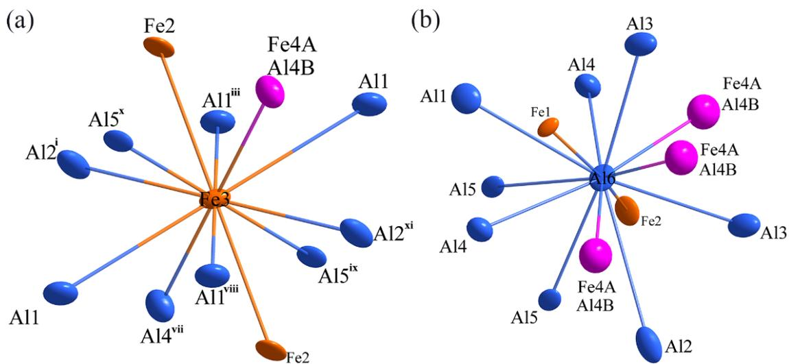
**Figure 5.** Environment diagram of atoms: (a) Fe3 atom; (b) Al6 atom. Symmetry codes: (i)  $-x, -y, -z + 1$ ; (iii)  $x - 1, y, z$ ; (vii)  $-x, -y, -z$ ; (viii)  $-x + 1, -y, -z$ ; (ix)  $-x, -y + 1, -z$ ; (x)  $x, y - 1, z$ ; (xi)  $x, y, z - 1$ .
