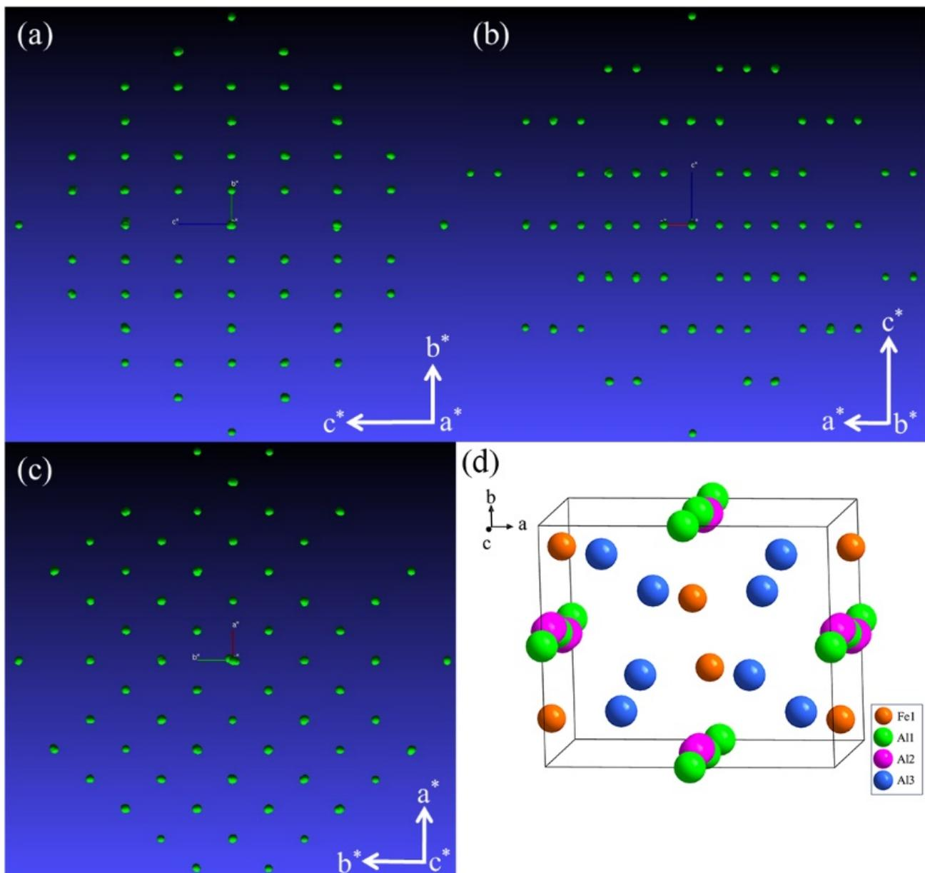
**Figure 3.** The diffraction patterns of the  $\text{Al}_5\text{Fe}_2$  and its crystal structure: (a) Projection along the  $a^*$ -axis; (b) Projection along the  $b^*$ -axis; (c) Projection along the  $c^*$ -axis; (d) Crystal structure of  $\text{Al}_5\text{Fe}_2$  phase.
