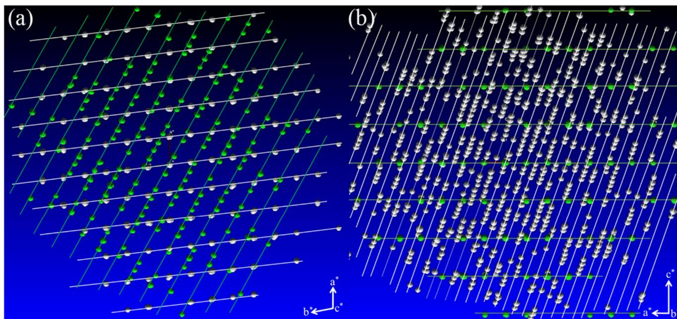
**Figure 1.** Diffraction points in the reciprocal space of the whole sample projected along different directions. The data set in white and green color indicates the  $\text{Al}_2\text{Fe}$  phase and the  $\text{Al}_5\text{Fe}_2$  phase, respectively: (a) Projection along the  $c^*$ -axis of the  $\text{Al}_2\text{Fe}$  phase; (b) Projection along the  $b^*$ -axis of the  $\text{Al}_5\text{Fe}_2$  phase.
