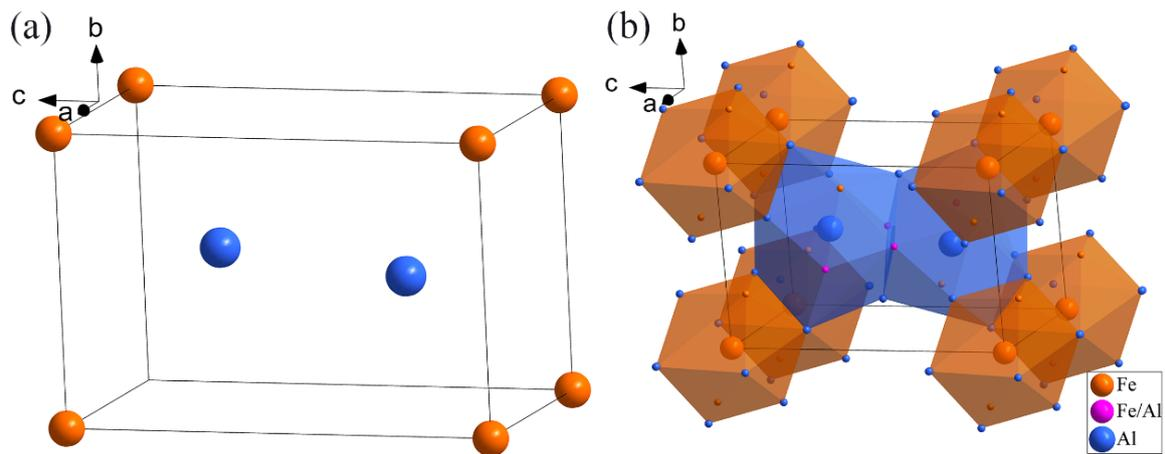
**Figure 4.** Cluster assembly in  $\text{Al}_2\text{Fe}$  phase cell: (a) The central atom of the cluster; (b) Cluster assembly model.
