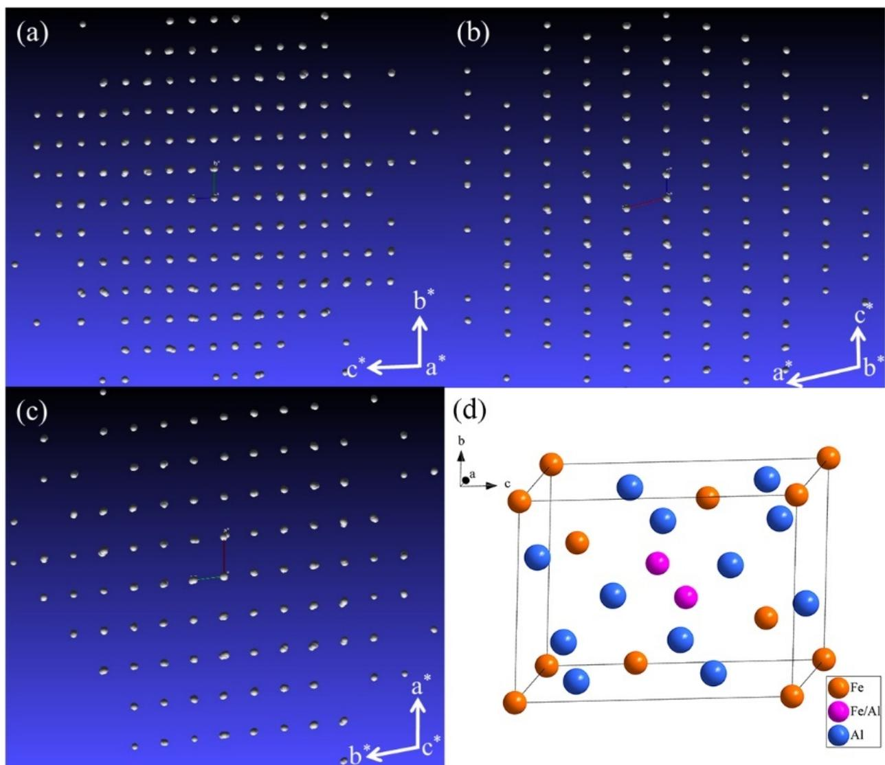
**Figure 2.** The diffraction patterns of the  $\text{Al}_2\text{Fe}$  and its crystal structure: (a) Projection along the  $a^*$ -axis; (b) Projection along the  $b^*$ -axis; (c) Projection along the  $c^*$ -axis; (d) Crystal structure of  $\text{Al}_2\text{Fe}$  phase.
