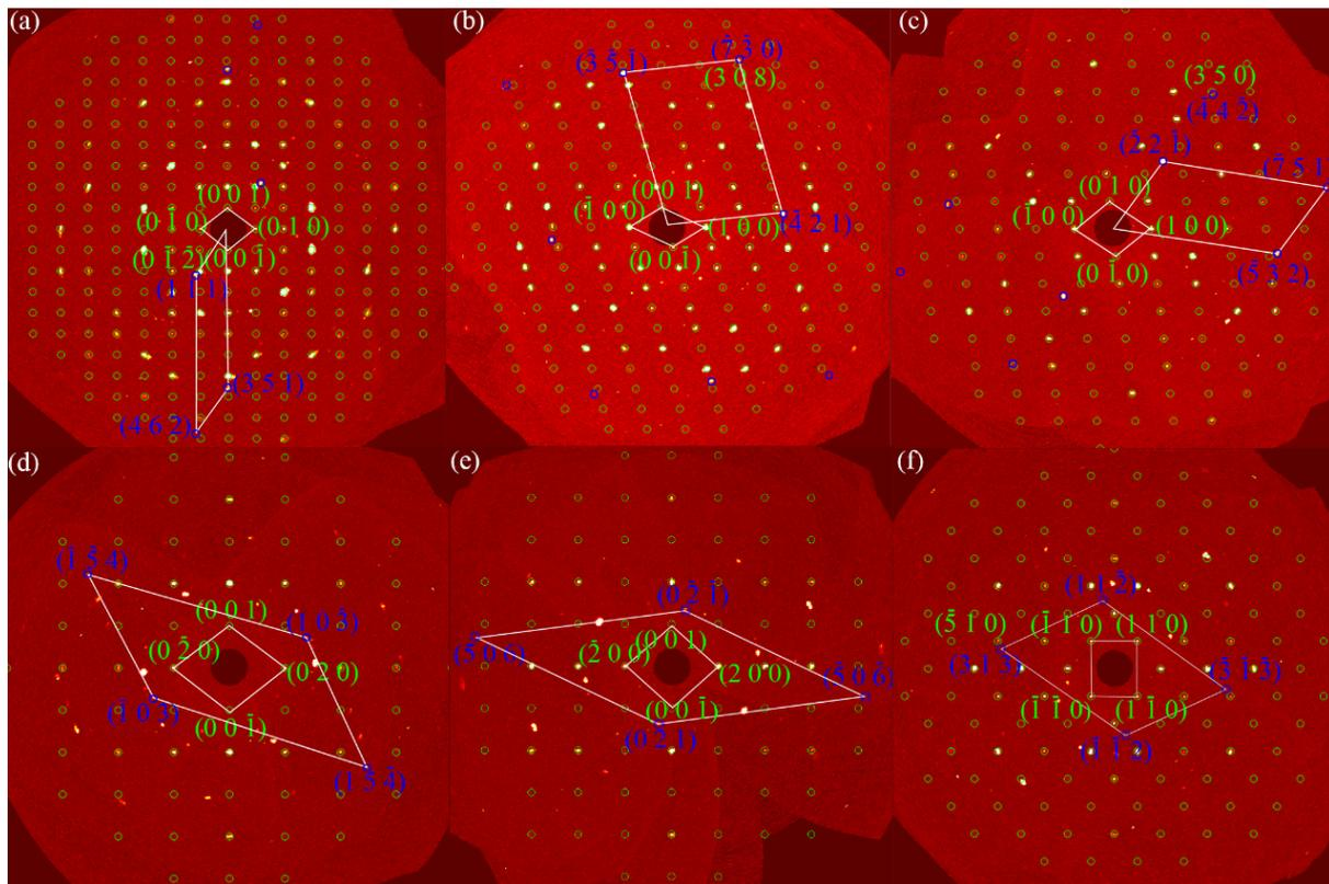
**Figure 9.** The precession images of intergrowth crystals: (a)  $\text{Al}_{12.48}\text{Fe}_{6.52}$  ( $0kl$ ), (b)  $\text{Al}_{12.48}\text{Fe}_{6.52}$  ( $h0l$ ), (c)  $\text{Al}_{12.48}\text{Fe}_{6.52}$  ( $hk0$ ), (d)  $\text{Al}_{5.72}\text{Fe}_2$  ( $0kl$ ), (e)  $\text{Al}_{5.72}\text{Fe}_2$  ( $h0l$ ), (f)  $\text{Al}_{5.72}\text{Fe}_2$  ( $hk0$ ).
