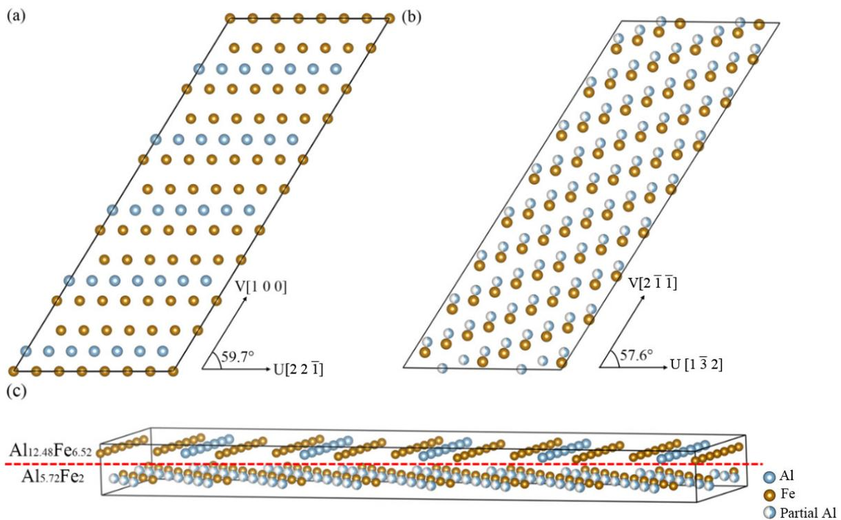
**Figure 10.** (a):  $\text{Al}_{12.48}\text{Fe}_{6.52} (01\bar{2})$  surface; (b):  $\text{Al}_{5.72}\text{Fe}_2 (111)$  surface; (c): the atomic interface model of  $\text{Al}_{12.48}\text{Fe}_{6.52} (01\bar{2})/\text{Al}_{5.72}\text{Fe}_2$ .
