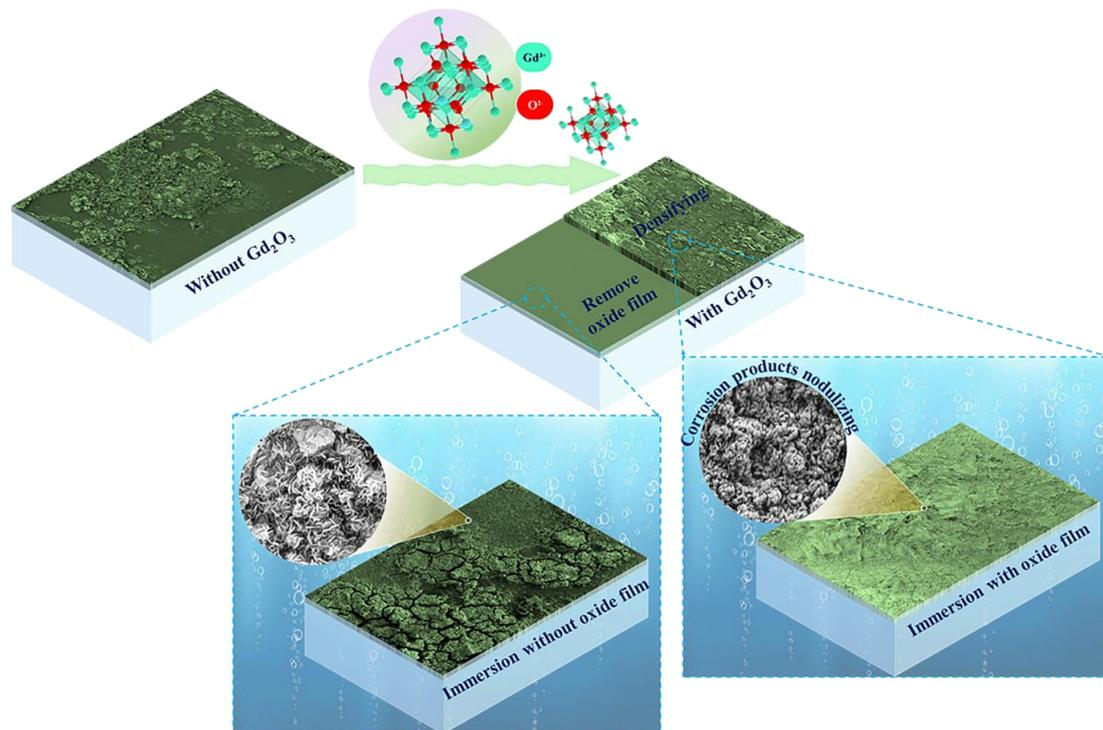
**Figure 14.** Schematic illustration of the mechanism of  $\text{Gd}_2\text{O}_3$  involvement in oxide film growth and nodulizing corrosion products.
