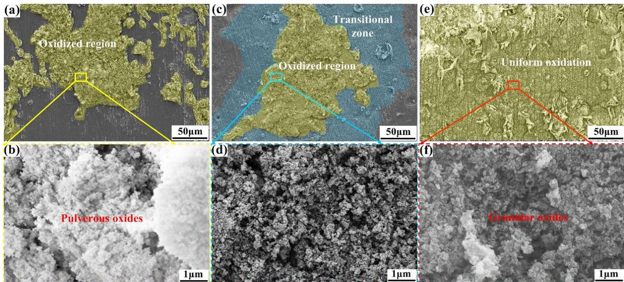
**Figure 5.** The micrographs of oxide films formed on the AZ80 (a,b), AZ80-0.47Gd (c,d), and AZ80-0.75Gd (e,f) alloys after 4.5 h of exposure at 420 °C.
