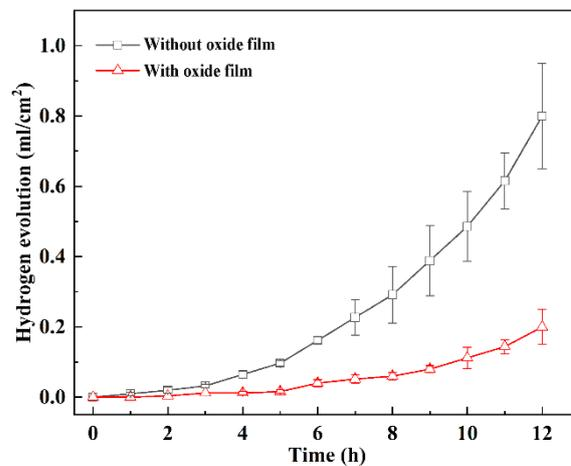
**Figure 12.** Hydrogen evolution curves of AZ80-0.75Gd samples with and without an oxide layer immersed in 3.5 wt% NaCl solution.
