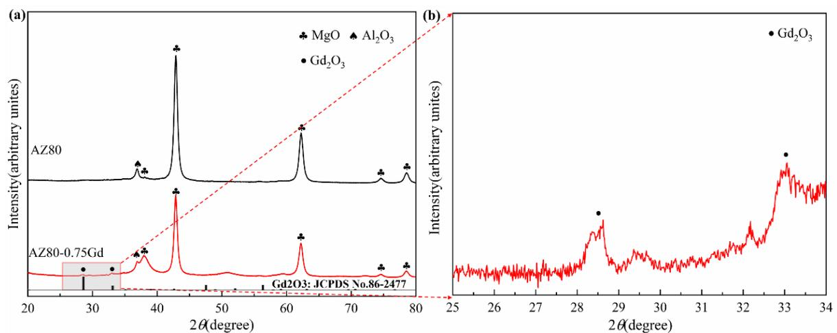
**Figure 7.** The normalized XRD patterns (a) and partially enlarged image (b) of the oxide products of the AZ80 and AZ80-0.75Gd alloys.
