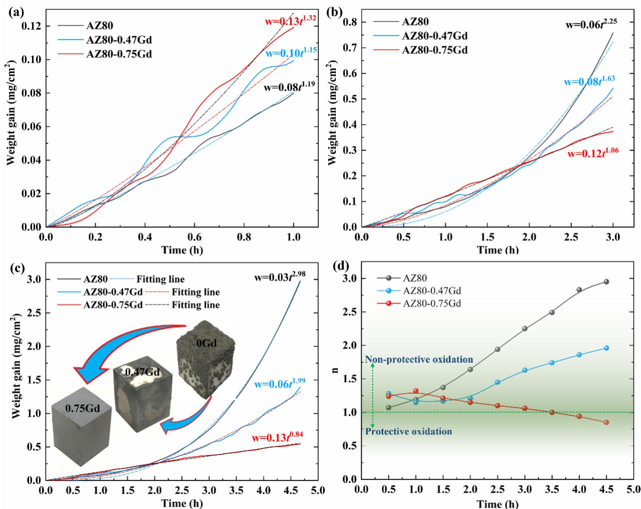
**Figure 3.** The weight gain behaviors of alloy oxidation for 1 h (a), 3 h (b), and 4.5 h (c) at 420 °C in air and the n values (d).
