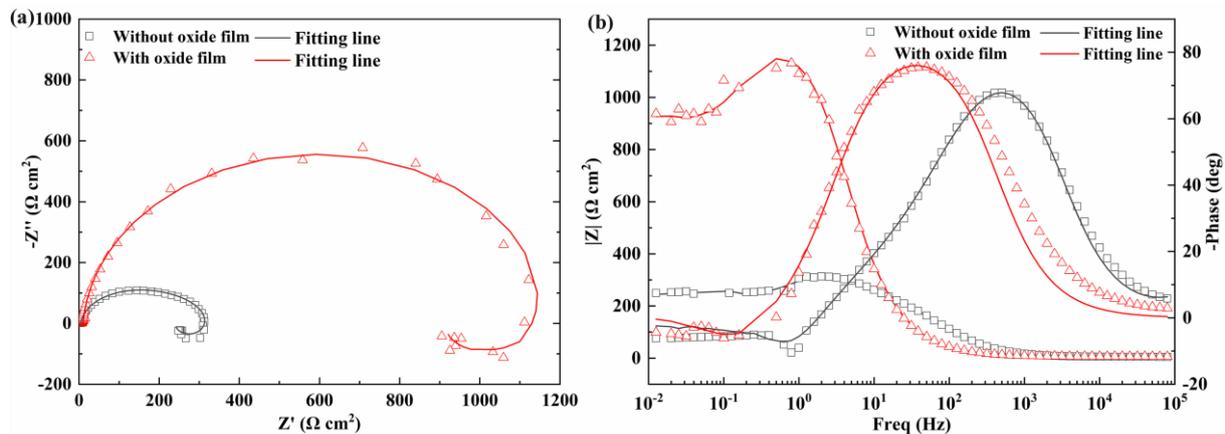
**Figure 10.** The EIS diagrams of the AZ80-0.75Gd samples after 1 h of soaking in 3.5 wt% NaCl solution: (a) Nyquist plots and (b) Bode plots of impedance modulus and phase angle.
