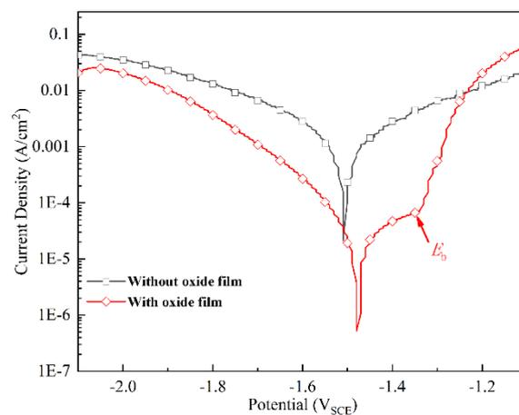
**Figure 9.** The potentiodynamic polarization curves of the AZ80-0.75Gd alloy with and without an oxide layer while soaking in 3.5 wt% NaCl solution for 1 h.
