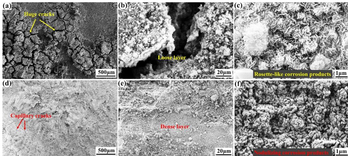
**Figure 13.** The microscopic corrosion morphologies of the AZ80-0.75Gd samples without (a–c) and with (d–f) an oxide layer after soaking for 12 h in 3.5 wt% NaCl solution.
