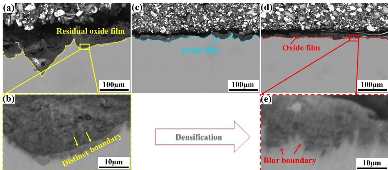
**Figure 6.** The cross-sectional microstructures of the AZ80 (a,b), AZ80-0.47Gd (c), and AZ80-0.75Gd (d,e) alloys after 4.5 h of exposure at 420 °C.
