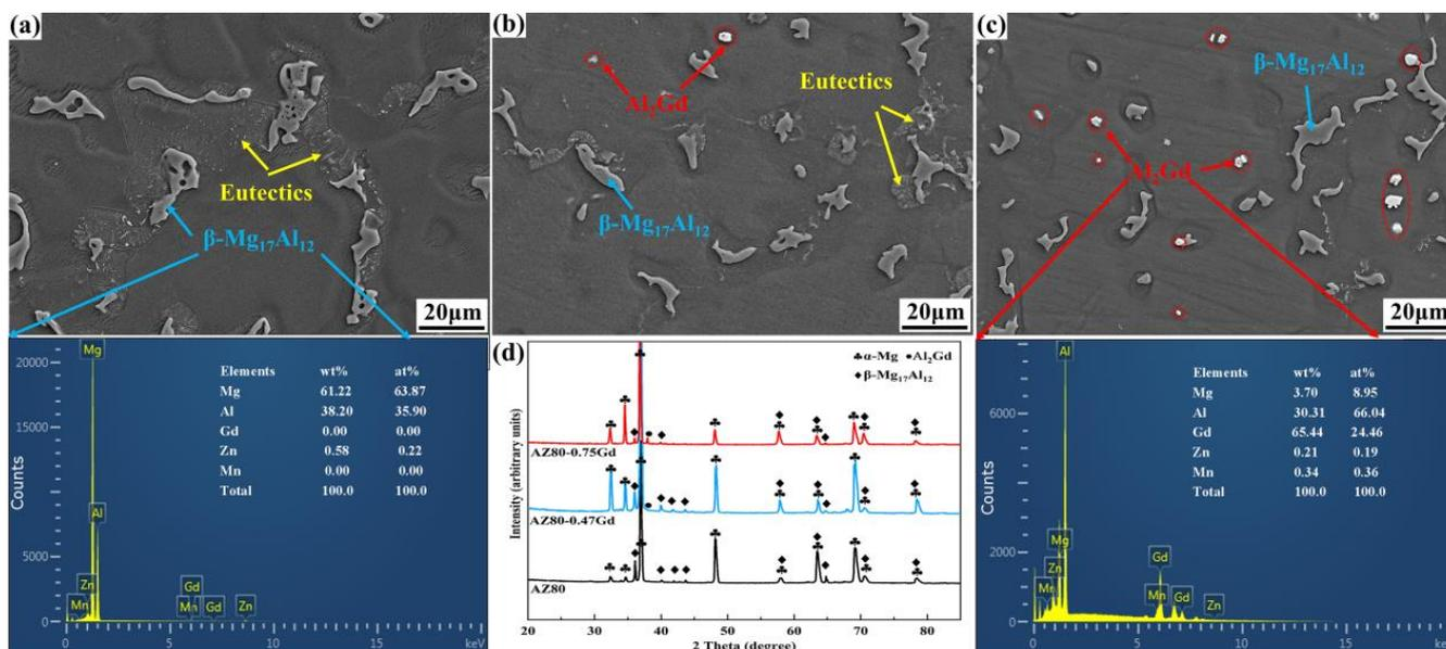
**Figure 1.** SEM microstructures of the AZ80 (a), AZ80-0.47Gd (b), and AZ80-0.75Gd (c) alloys with  $\beta$ -Mg<sub>17</sub>Al<sub>12</sub> and Al<sub>2</sub>Gd phases energy dispersive X-ray spectroscopy analysis as well as normalized X-ray diffraction patterns (d).
