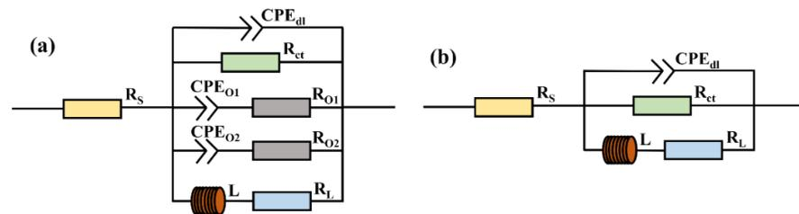
**Figure 11.** Equivalent electrical circuits used for the simulation of EIS data in Figure 10: (a) sample without oxide film and (b) sample with oxide film.
