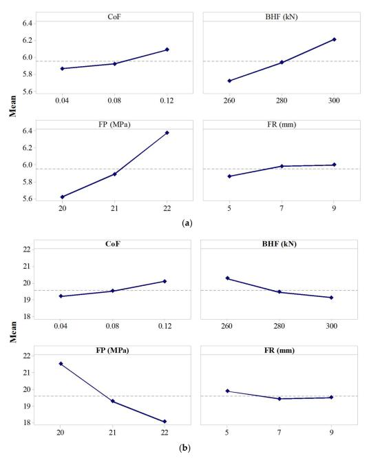
Figure 10. (a) Main effect plot for a thinning percentage. (b) Main effect plot for corner radius.
