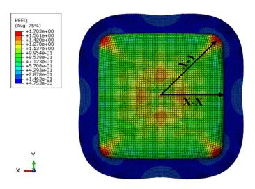
**Figure 7.** Fully formed cup depicting X-X and X-Y direction.
