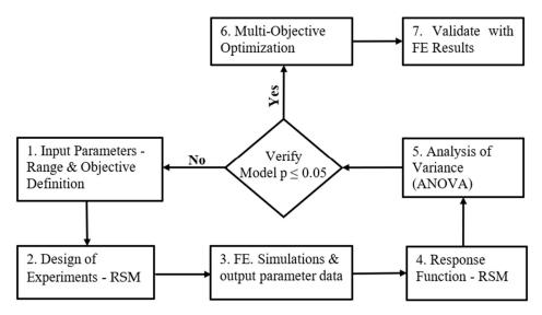
Figure 6. Optimization Process Flow Chart.
