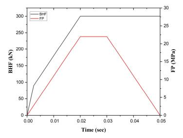
Figure 5. Loading and unloading FP path and BHF vs. time.
