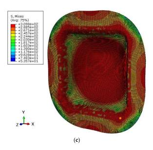
**Figure 9.** (a) Von Mises stress distribution in fully formed cup at 22 MPa peak FP. (b) Equivalent plastic strain in fully formed cup at 22 MPa peak FP. (c) Von Mises stress distribution in partially formed cup at 18 MPa peak FP.
