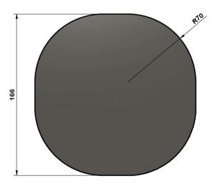
Figure 2. Blank Geometry and Dimensions.
