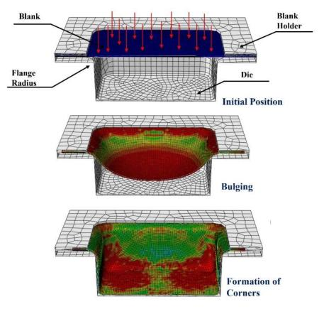
Figure 1. Various stages of the CDSHF process of a square cup using FE modeling.
