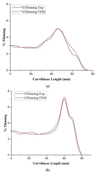
**Figure 8.** (a) Comparison of % thinning in X-X direction. (b) Comparison of % thinning in X-Y direction.
