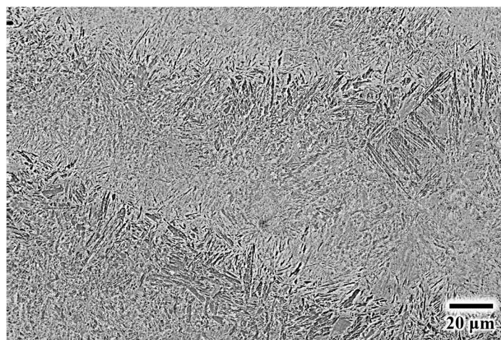
Figure 11. Backscatter electron micrograph of typical alternating fine and coarse martensite layers in as-fabricated 4340 steel.
