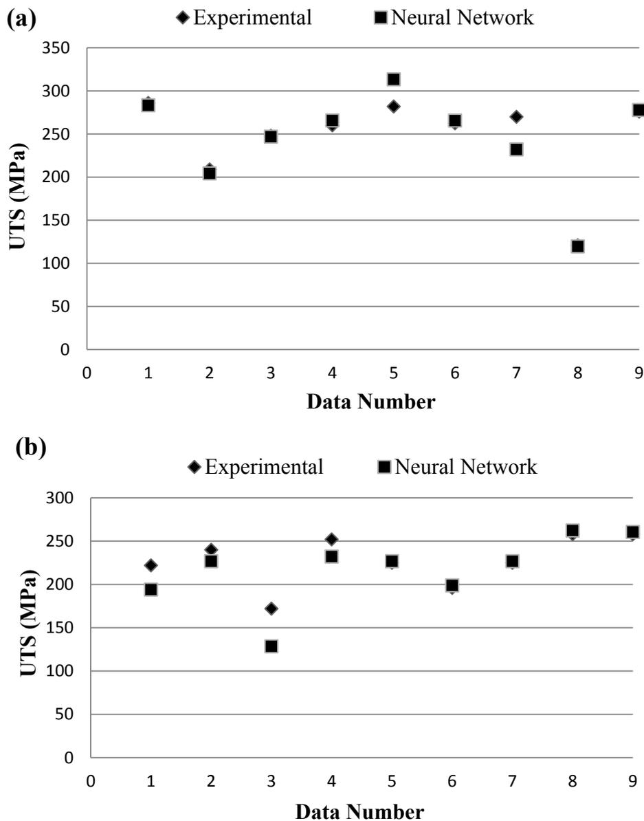
**Figure 2.** Correlation of neural network (NN) and experimental results for (a) validation and (b) test sets.
