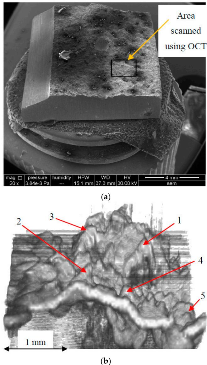
**Figure 9.** Images of a fracture in an OLC 45 steel: (a) SEM overview of the entire sample, with the marked area for OCT imaging; (b) OCT image of the selected area, obtained with the MS/SS-OCT system with the improved 4  $\mu\text{m}$  transversal resolution, with several grains numbered on the surface.
