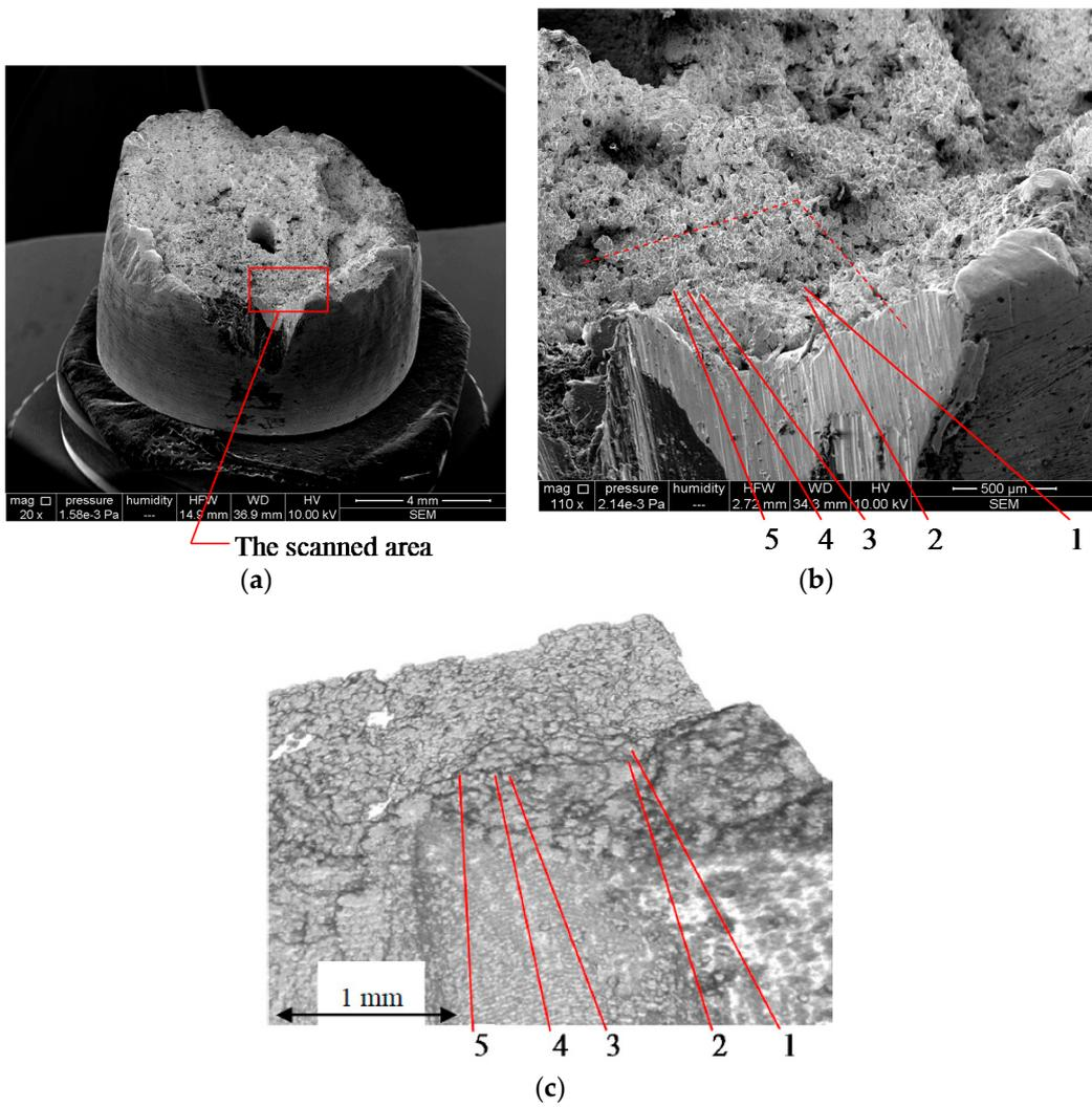
**Figure 7.** Images of a fracture in a Sn-Sb-Cu antifriction alloy: (a) frontal SEM overview of the entire sample, with a marked area for the OCT investigation; (b) SEM image of the selected area; (c) OCT image of the same area with a 10  $\mu\text{m}$  transversal resolution, with the same grains as in (b) numbered on the surface.
