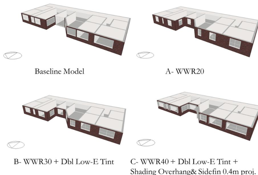
**Figure 12.** Illustrations of the highest-performing evidence-based design options for the west façade energy optimization.
