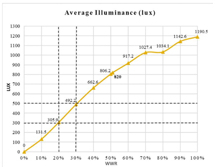
**Figure 7.** Effect of west façade WWR on the average illuminance (lux) in a typical office.
