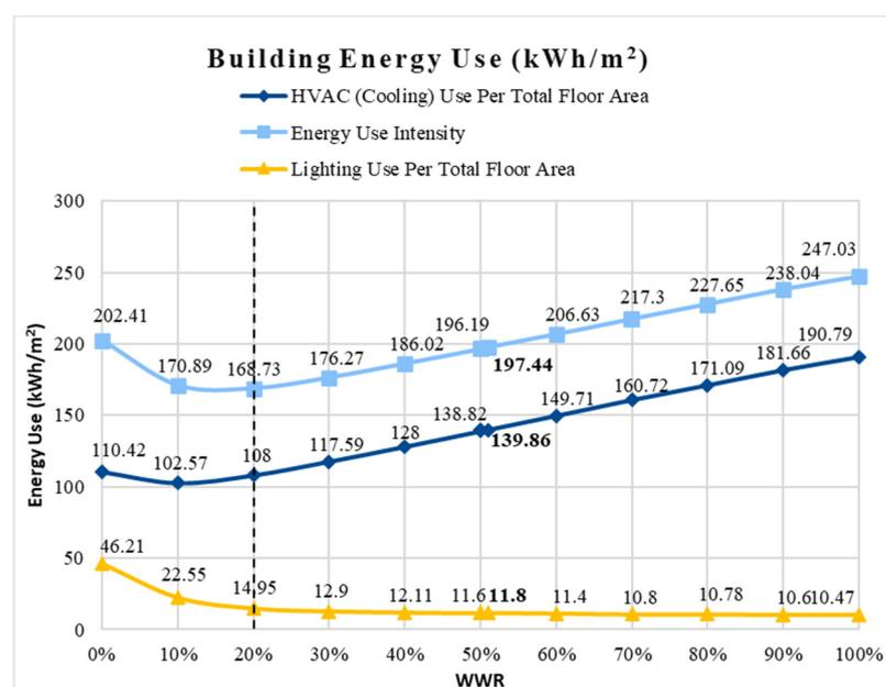
**Figure 6.** Effect of west façade WWR on building energy use per total floor area (baseline simulation values highlighted in bold).
