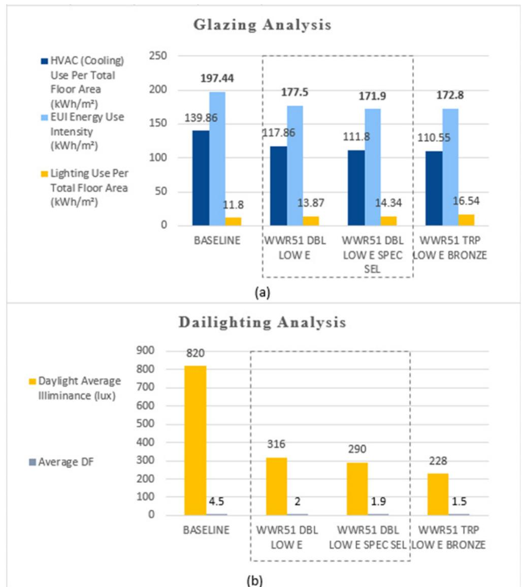
**Figure 8.** Effect of glazing type on building energy use (a) and daylight illuminance (b) (optimum performance highlighted in the dotted box).
