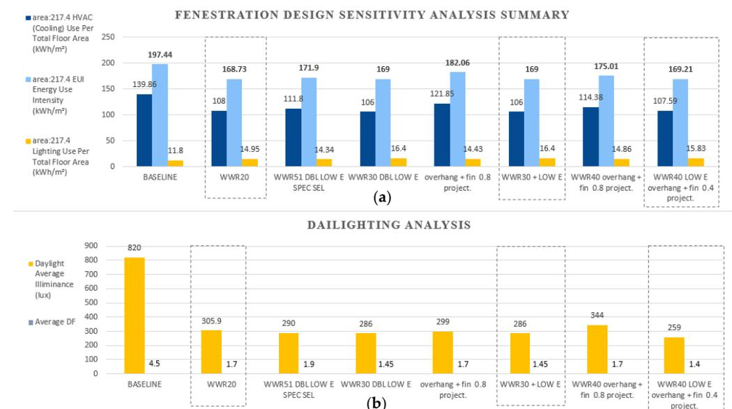
**Figure 11.** Summary of the highest performing results of WWR, glazing types, and external shading options in terms of the total building energy use (a) and daylighting levels (b) on the west façade (optimum performance highlighted in dotted box).
