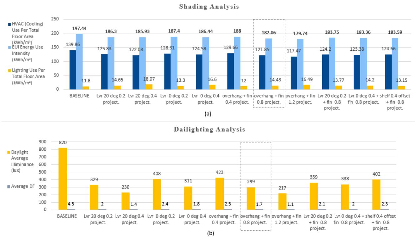
**Figure 9.** The effect of different external shading options on the total building energy use (a) and daylighting levels (b) of the west façade (best performance highlighted in dotted box).
