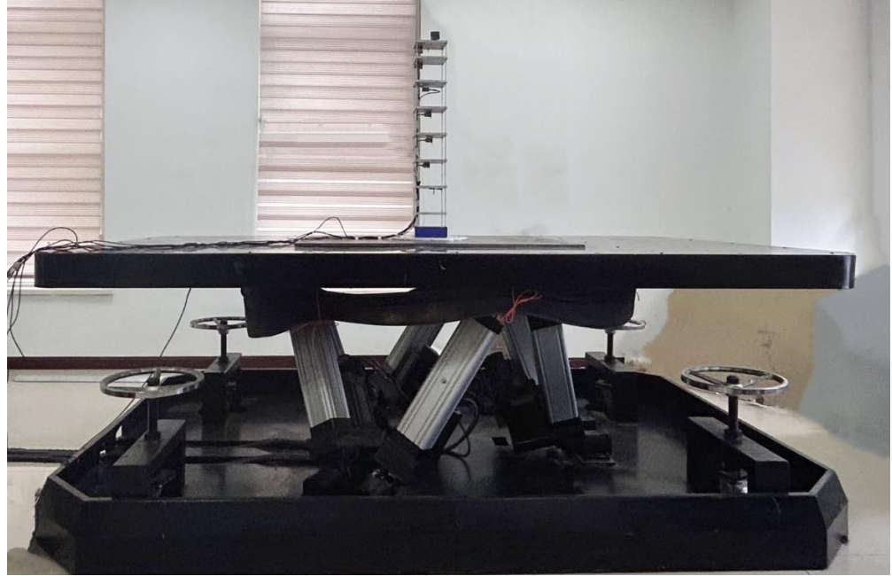
Figure 6. The model installed on the shake table.
