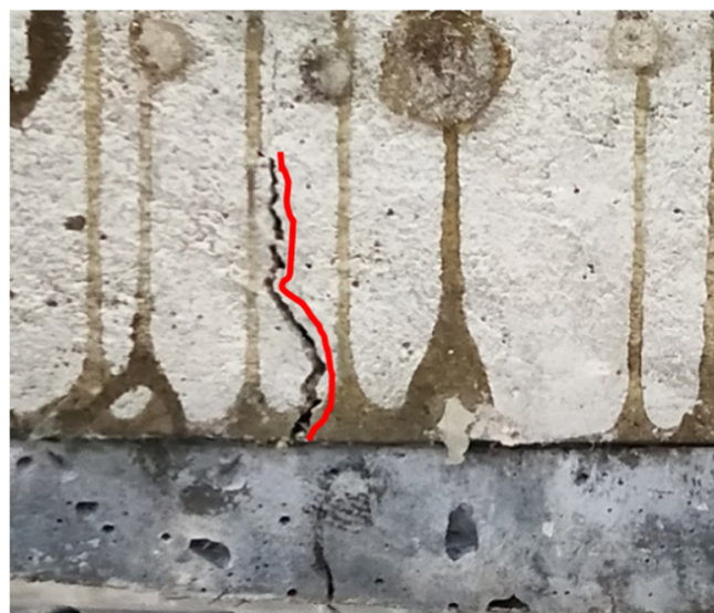
Figure 10. Damage mode of bonded group specimens.
