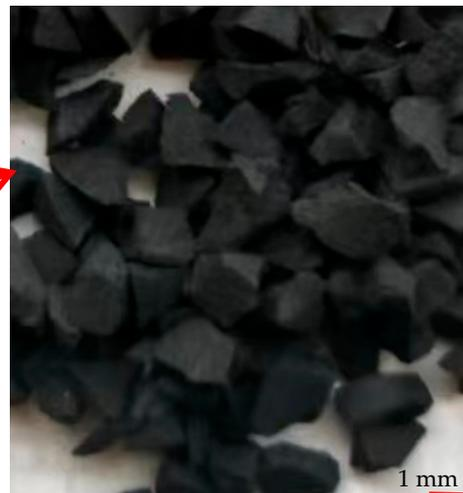
(b) Rubber particle enlargement diagram.
