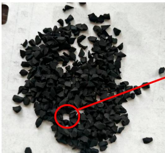
(a) Figure of accumulation of 30-mesh crumb rubber aggregate.
