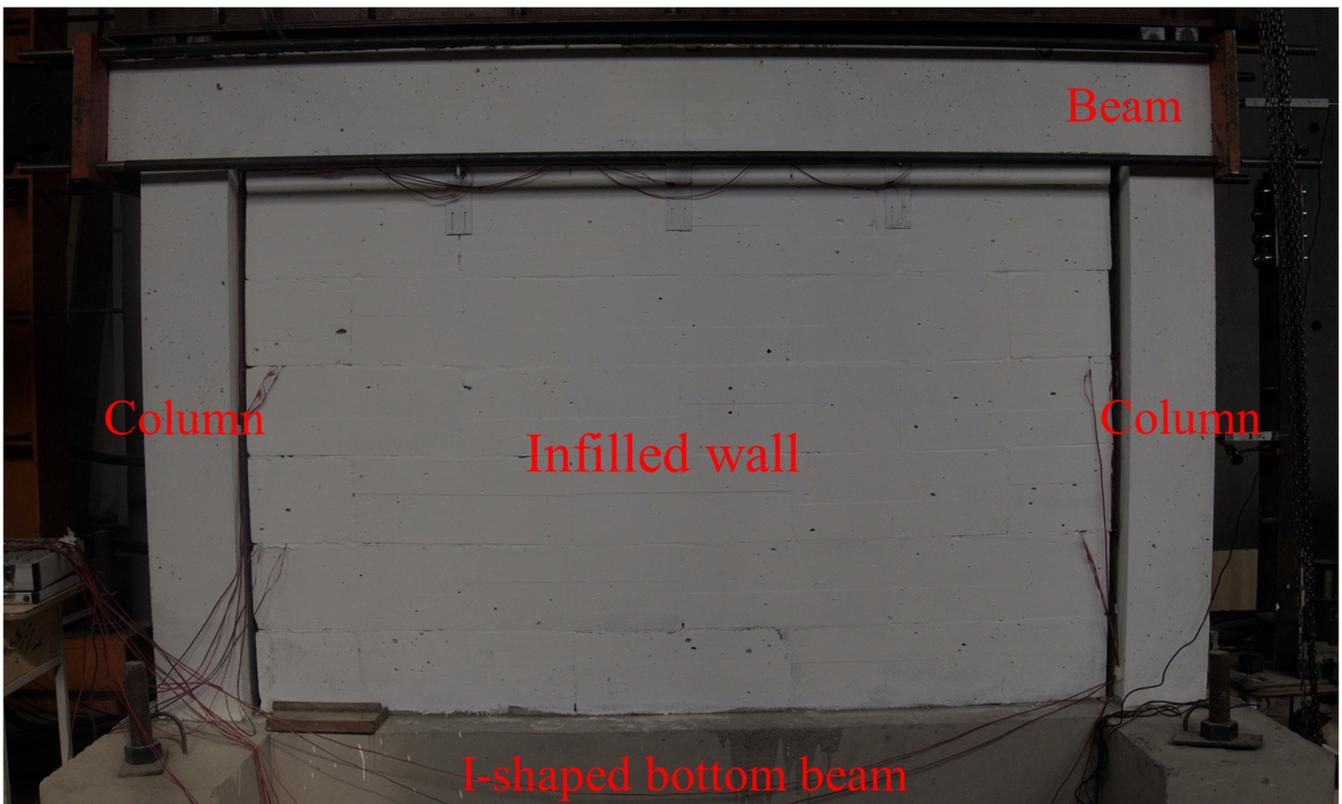
**Figure 1.** The frame and infilled wall schematic.
