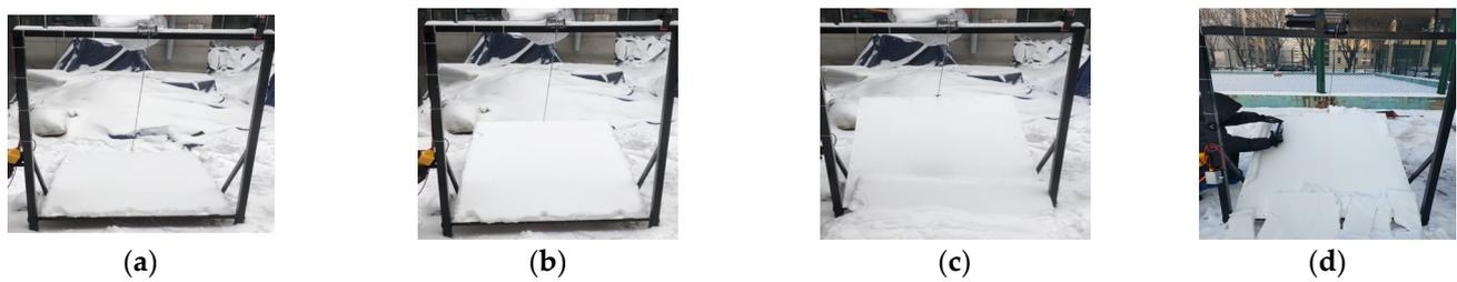
**Figure 3.** Test process of the critical angle tests for roof snow sliding: (a) place the specimen on the test platform; (b) rotate the roof model slowly; (c) stop rotating when the snow slides; (d) measure the roof angle.
