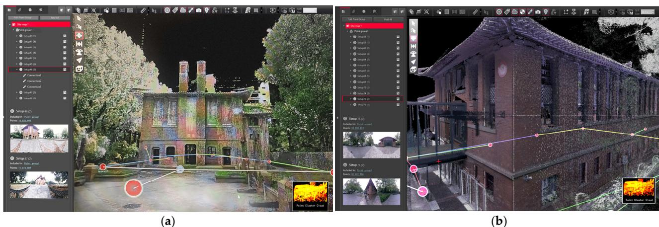
**Figure 8.** Preprocessed point cloud data result map (source: author). (a) North facade point cloud data. (b) Southeast facade point cloud data.
