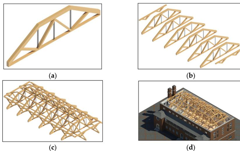
**Figure 10.** Three-dimensional model of beam frame family (source: author). (a) A roof truss. (b) Multiple roof trusses. (c) Tandem roof trusses. (d) Arrangement of roof trusses.
