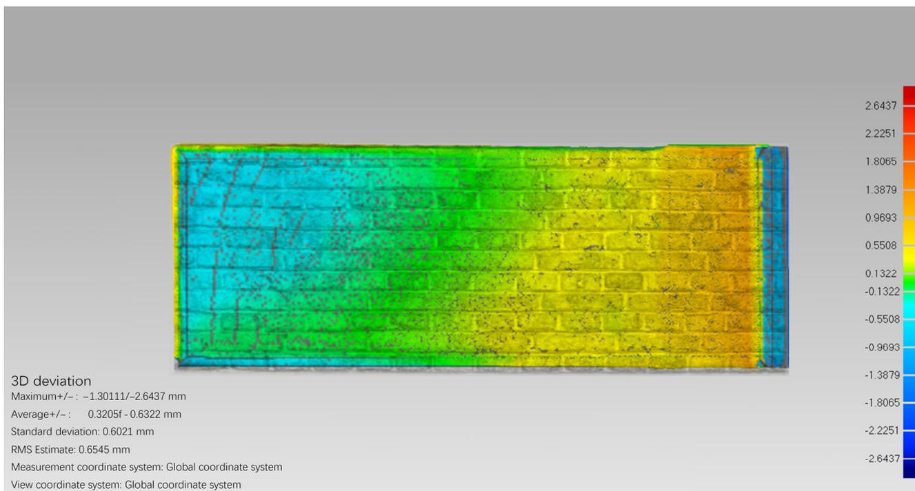
**Figure 18.** Analysis of Building Surface Elevation Deviation (source: author).
