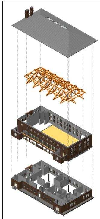
Figure 11. Disassembly drawing of building components (source: author).
