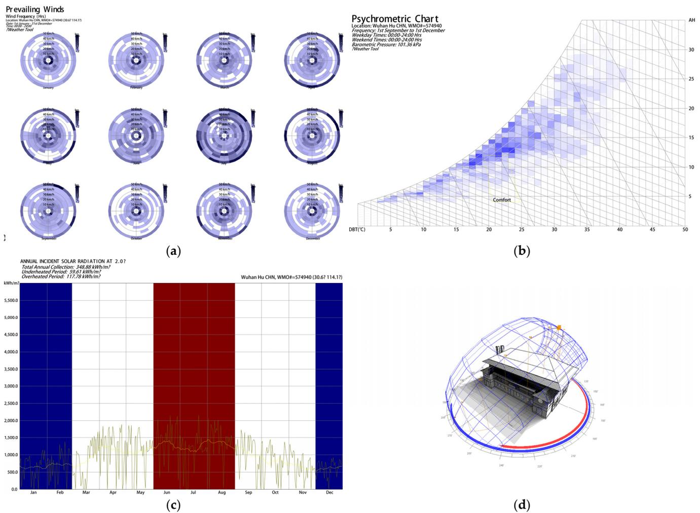
**Figure 17.** Environmental simulation analysis in Wuhan area (source: author). (a) Wind environment simulation. (b) Enthalpy and humidity analysis. (c) Analysis of due-north solar radiation. (d) Shadow distribution on the winter solstice.
