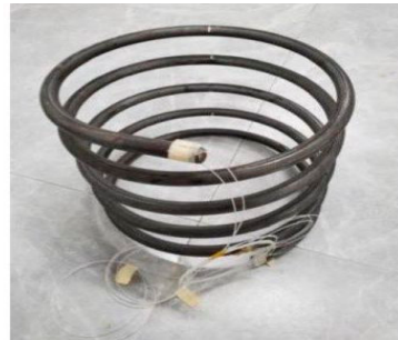
Figure 21. Real picture of FBG spiral reinforcement.
