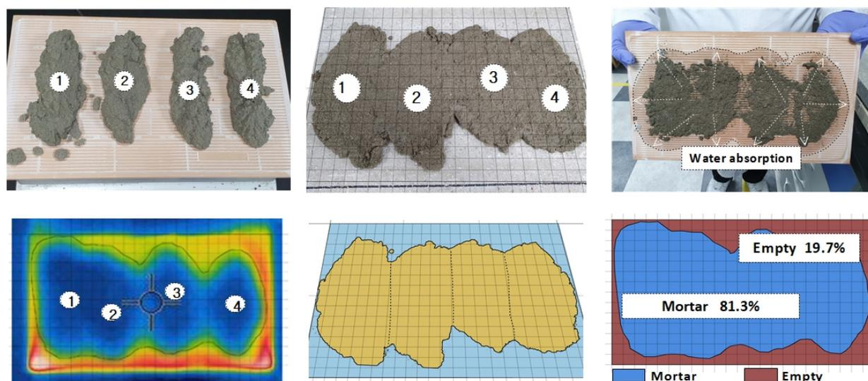
**Figure 4.** Observation and area calculation after mortar construction.
