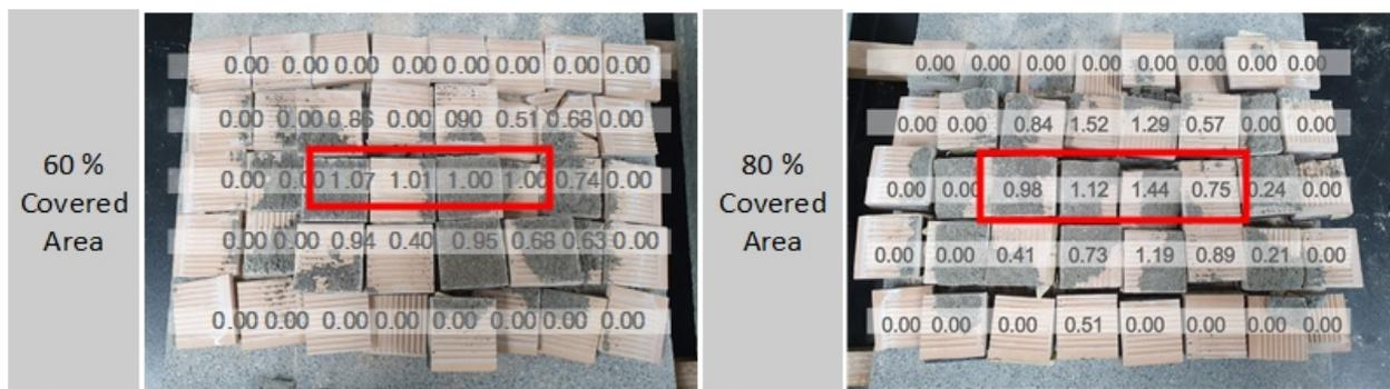
**Figure 12.** Current status of comparative specimens with 60% and 80% covered area (Red box: where the adhesion strength is highest).
