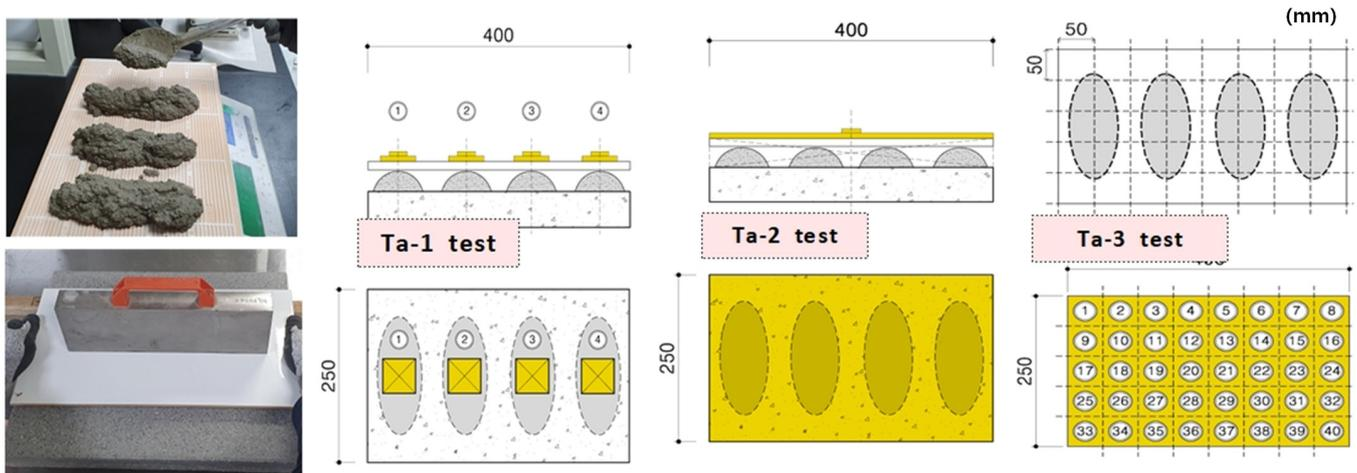
Figure 5. Attachment stability test status (mm) according to mortar attachment area from Table 2.
