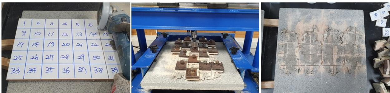
**Figure 11.** Status of partial adhesion strength test after cutting for whole tile.
