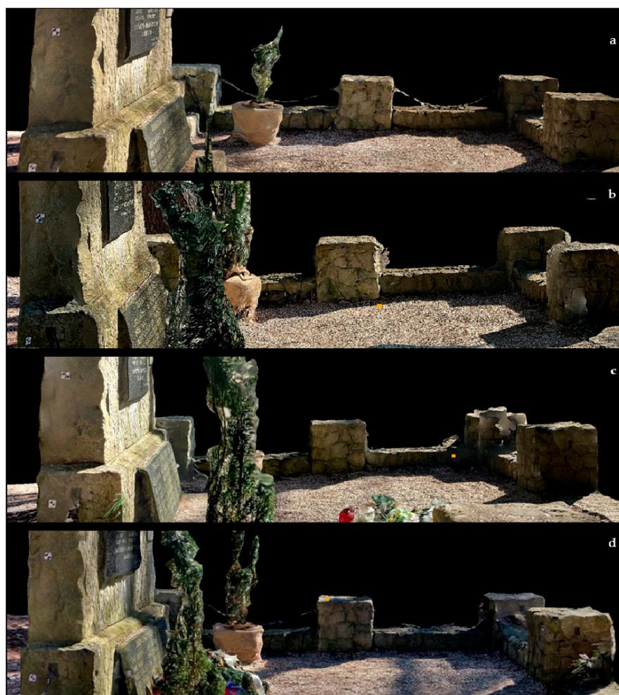
**Figure 11.** Focusing on the challenging components capture abilities of (a) Scaniverse, (b) 3DScanner-App, (c) Polycam—LiDAR approach, (d) Polycam—photogrammetry approach.
