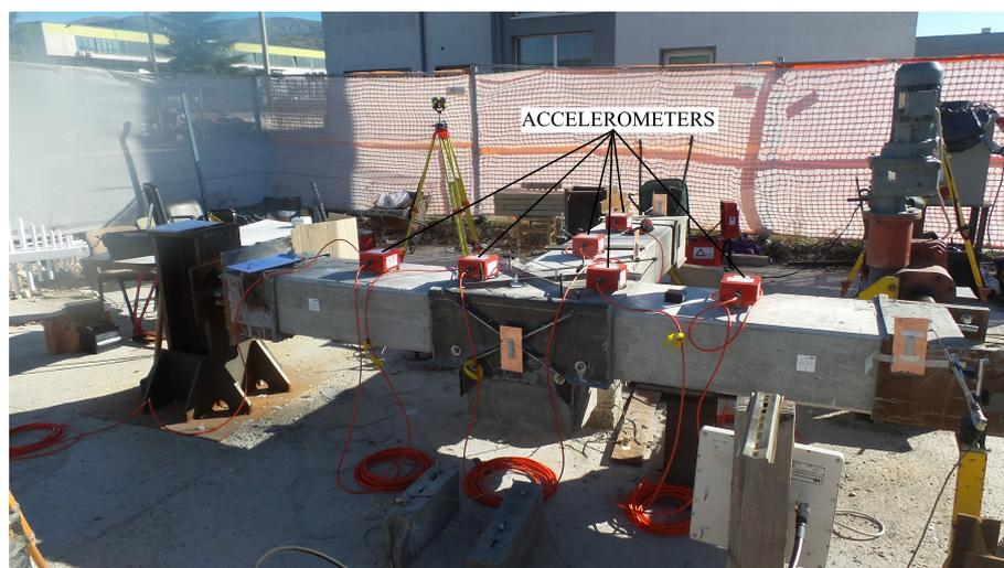
**Figure 3.** Experimental layout with a view of the measuring devices.
