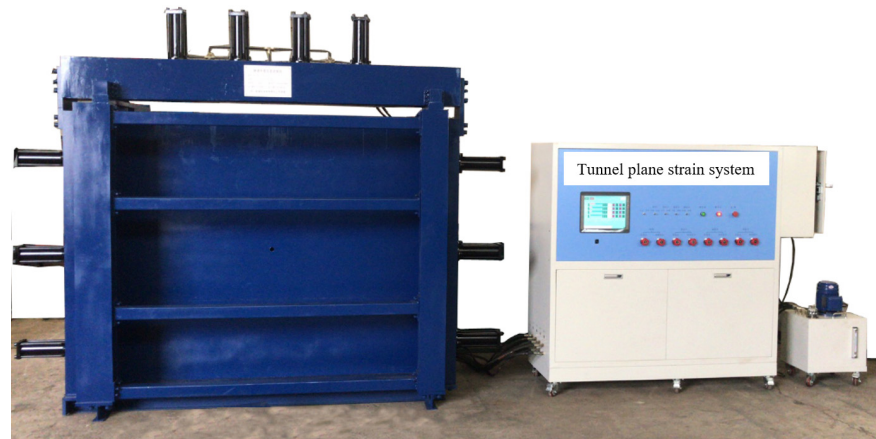
Figure 2. Model test equipment, control systems, and loading systems.
