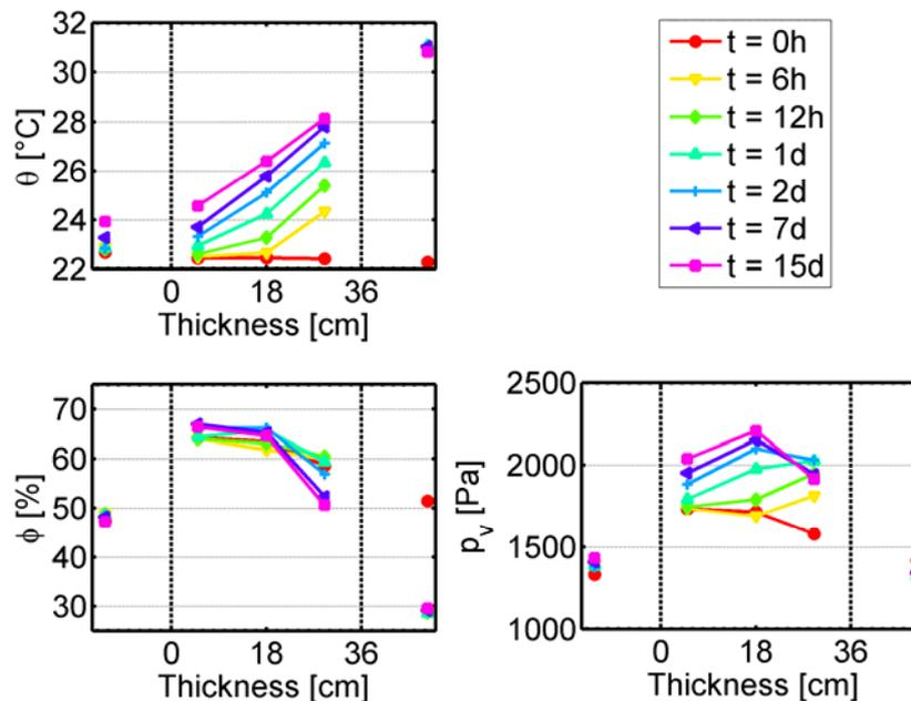
On the other hand, the vapor pressure increases during the first days ( $t < 5$  d) on the outdoor side ( $x = 29$  cm): this may be attributed to evaporation and molecular desorption. Indeed, for given temperature and relative humidity, capillary condensation occurs in pore with a radius  $r$  given by the Kelvin-Laplace equation:
