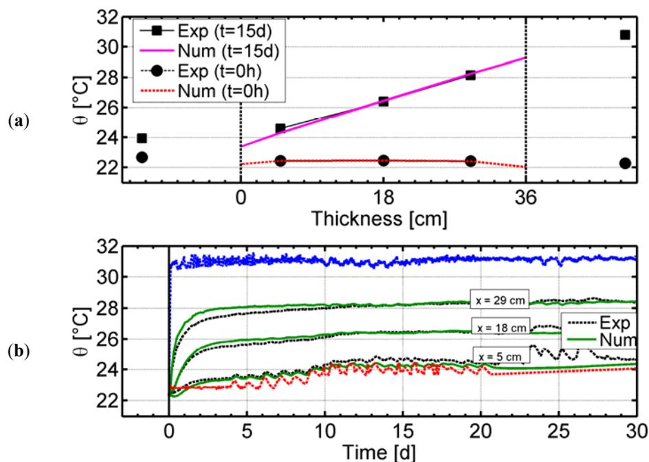
**Figure 11.** Sensitivity analysis (colored lines) to the thermal properties (see Table 3) and comparison to experimental results (black lines). Top graph (a) shows the spatial response at  $t = 15$  d; bottom graph (b) the transient response at  $x = 18$  cm.
