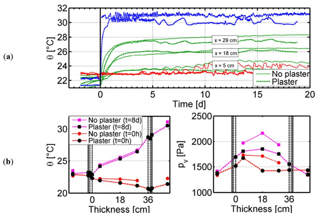
Figure 14 allows comparing experimental and numerical results. Thermal properties used for the simulation are summarized on Table 4. As in Figure 10, the steady state temperature profiles overlay perfectly. Transient evolution of temperature is also well caught, even for the indoor and the outdoor
