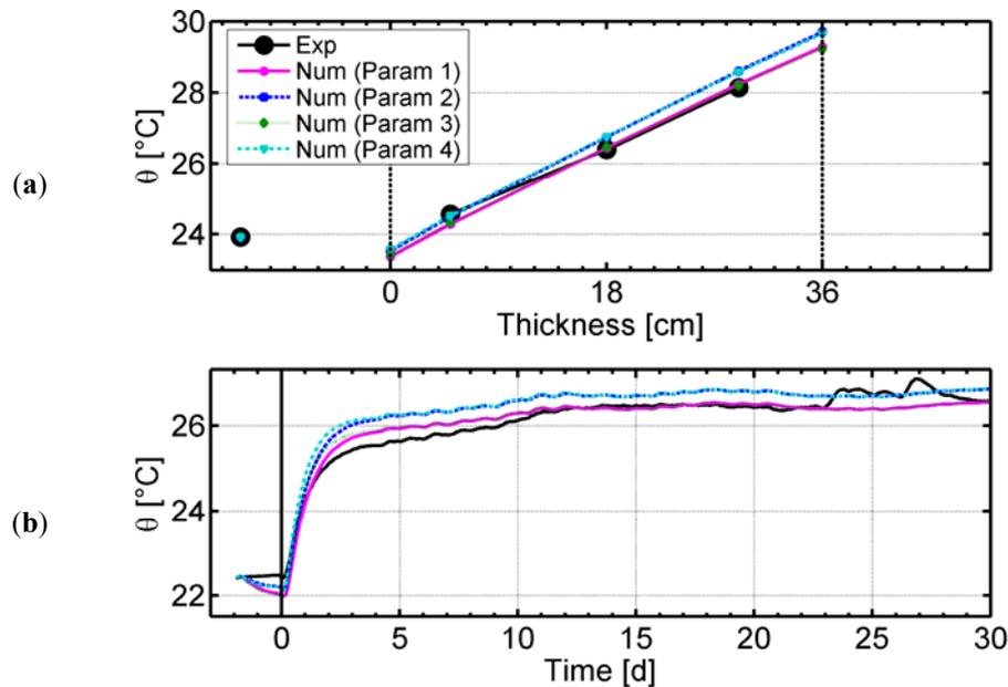
Finally, numerical and experimental results of Experiment 2 are presented in Figure 12. Globally, we observe that the numerical results are also lower than the experimental ones, but profiles at steady state are parallel.
