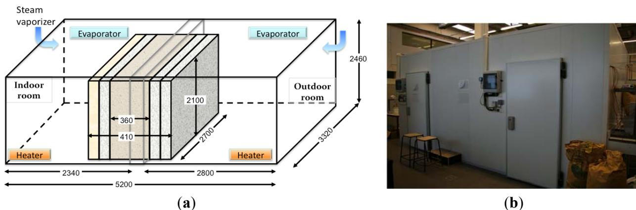
Each room is insulated from the laboratory with polyurethane panels ( $U \approx 0.4 \text{ W}\cdot\text{m}^{-2}\cdot\text{K}^{-1}$ ) and equipped with heating, refrigeration (for cooling or dehumidifying) and moisture control equipment (steam vaporizer) to maintain temperature and relative humidity to the desired level (see Figure 1a). Controllers (type DR4020 from Eliwell) are used to fix the set points. Working range and accuracy of the set-up are given in Table 1.
