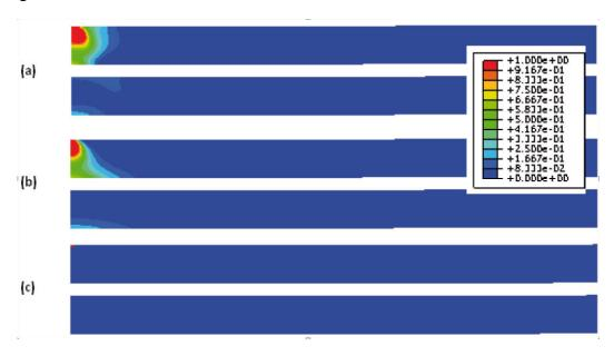
**Figure 5.** Contour plots of damage in laminated glass at 3.4 ms after impact for large missile with round end configuration: (a) web-shaped damage  $D_{11}$ ; (b) star-shaped damage  $D_{33}$ ; (c) shear damage  $D_{12}$ .
