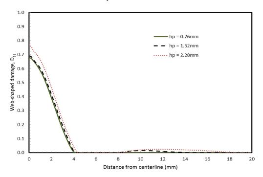
**Figure 9.** Effect of PVB interlayer thickness on web-shaped damage,  $D_{11}$  on surface S4 for large missile (round end) impact.
