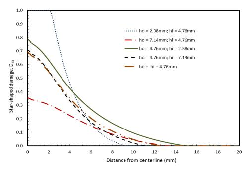
**Figure 12.** Effect of inner and outer plies thickness on Damage variable  $D_{11}$  (web-shaped) at surface S4 for large missile (round end) impact.
