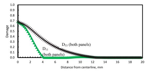
**Figure 15.** Effect of panel area on Damage variables  $D_{11}$  (web-shaped),  $D_{33}$  (star-shaped) at surface S4 for large missile (round end) impact.
