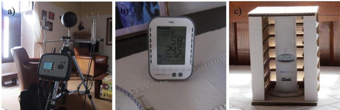
**Figure 3.** (a) Thermal microclimate station; (b) thermo-hygrometer + datalogger; (c) thermo-hygrometer sensor.
