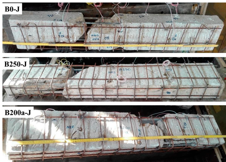
Figure 6. Heavily shear-damaged beams after concrete surface preparation (cleaning and roughening) and the installation of the jacketing reinforcement.
