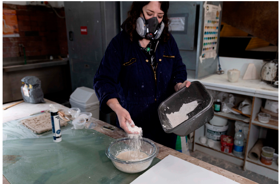
Figure 18. Longwill creating plaster/silica molds for glass. Photo by Joe Lington.
