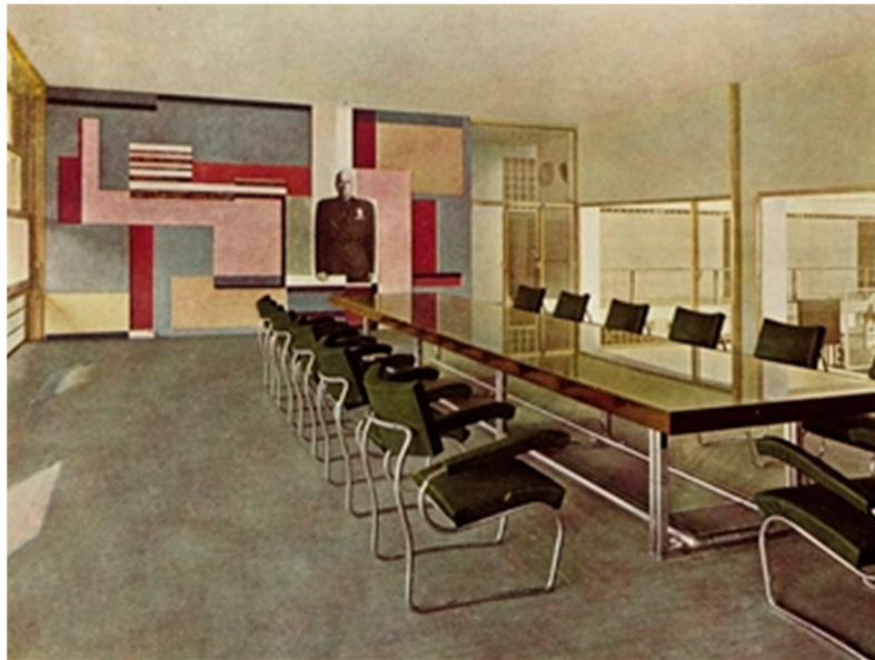
Figure 25. Casa del fascio by Giuseppe Terragni. Como (1932–1936). Directory room, table in chromed alpaca stiffened with anticorodal tubular. Top protected by glass sheet 140 cm × 700 cm, thickness 10 mm. Fresco by Mario Radice. Armchairs model “Benita”. Table and armchairs produced by the company Columbus. Photo from ( Sartoris 1941 , p. 398).
