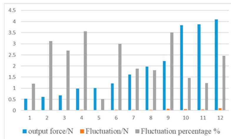
**Figure 13.** Output force and its fluctuation when the bottom of haptic device is fixed.
