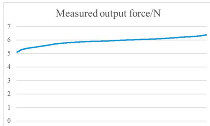
**Figure 17.** Measured output force while the constant force is 6 N along z axis.
