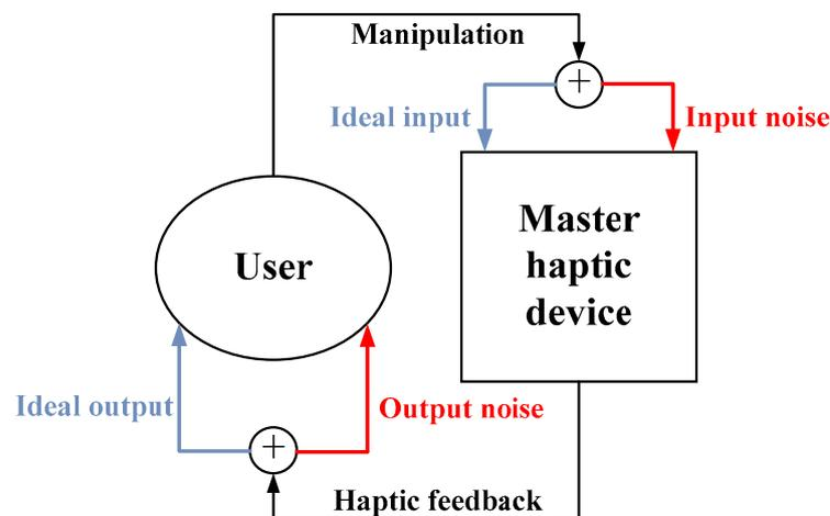
Figure 2. Relationship between human user and master haptic device in teleoperation.
