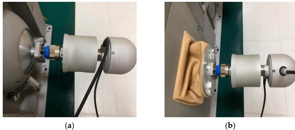
**Figure 14.** iGrasp-R and iGrasp-T manipulated by a user. (a) iHandle install at the end of iGrasp-R; (b) iHandle install at the end of iGrasp-T.
