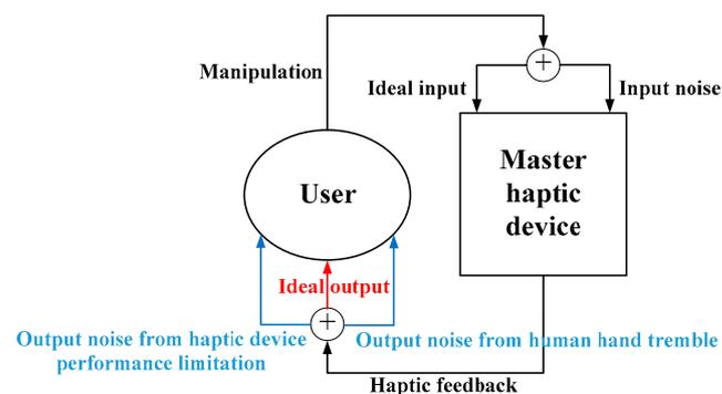
Figure 19. Analysis of the input noise and output noise of haptic based teleoperation.
