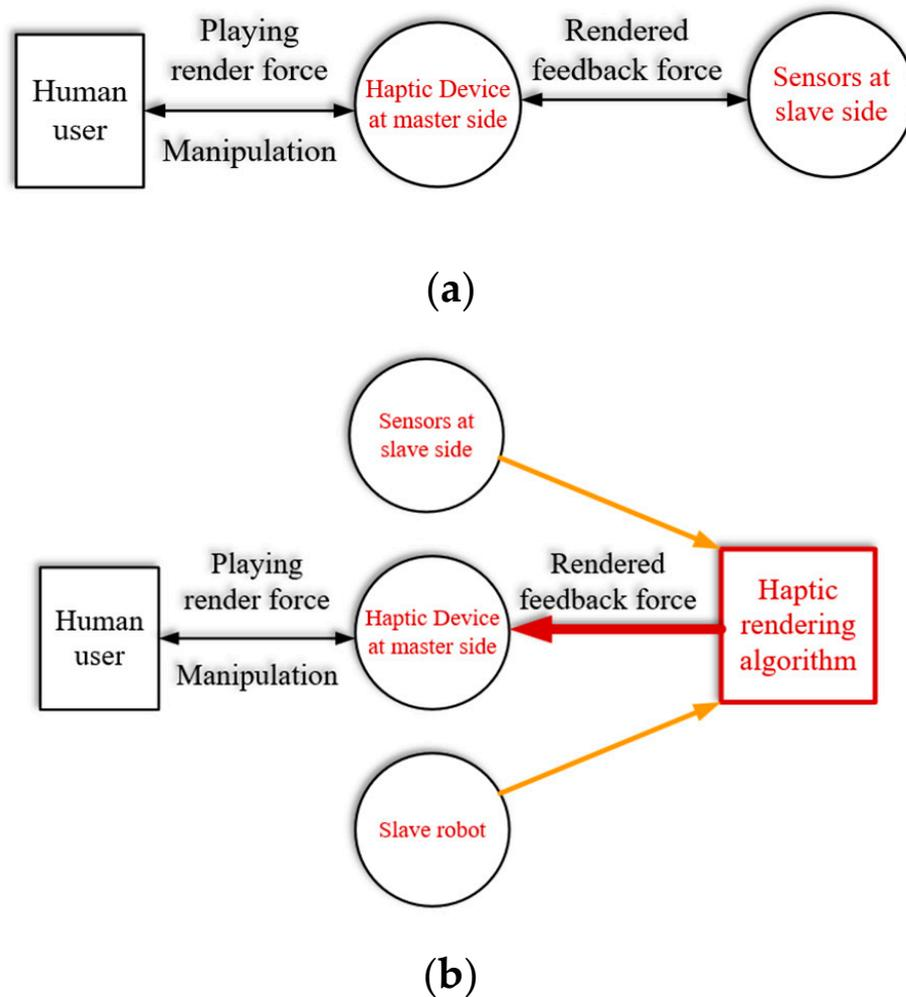
**Figure 18.** Two types of haptic rendering algorithms for haptic based teleoperation (a) Direct record and play; (b) Indirect rendering based on measured data.
