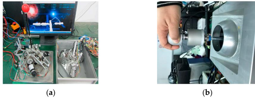
**Figure 9.** (a) Two haptic devices designed for robotic teleoperation; (b) haptic device with iHandle.
