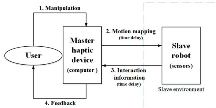
Figure 1. Description of block diagram of haptic based teleoperation.
