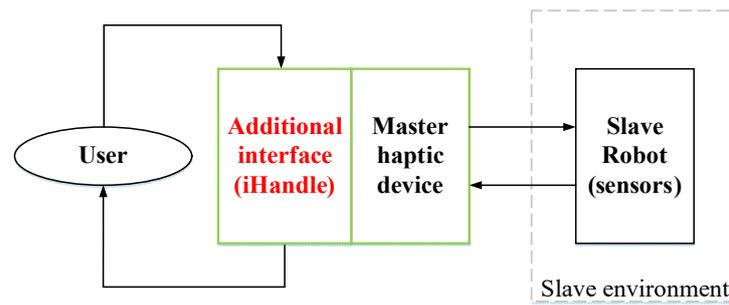
Figure 3. Description of block diagram of haptic based teleoperation.
