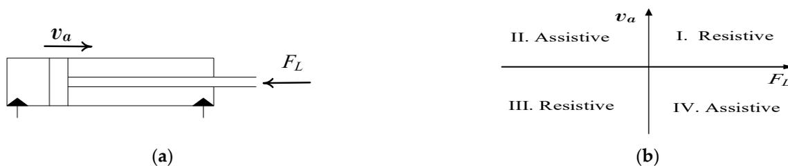
**Figure 1.** Single-rod cylinder: (a) sign convention; (b) quadrants of operation.
