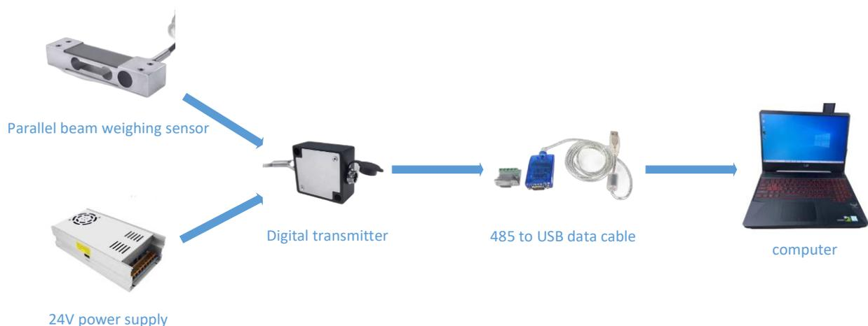
**Figure 7.** Schematic diagram of load cell experiments.
