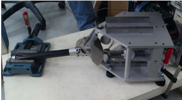
**Figure 14.** Configuration used to measure the transmission stiffness.
