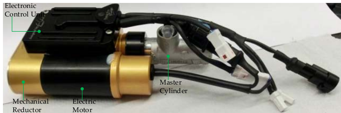
(a) Prototype of hybrid brake-by-wire actuator
