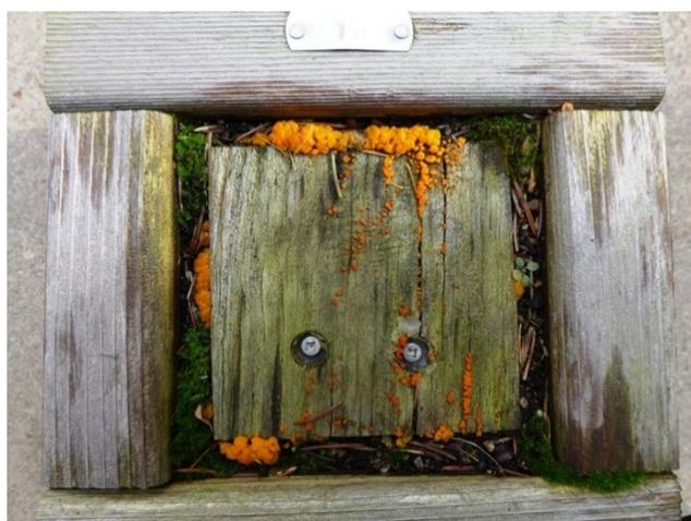
**Figure 2.** Visual example of untreated pine block at the end of the test. Note moss growth indicative of high moisture content and surface growth of saprophytic fungi on the surface of the block, presumably *Dacrymyces* spp. (likely *capitatus*).
