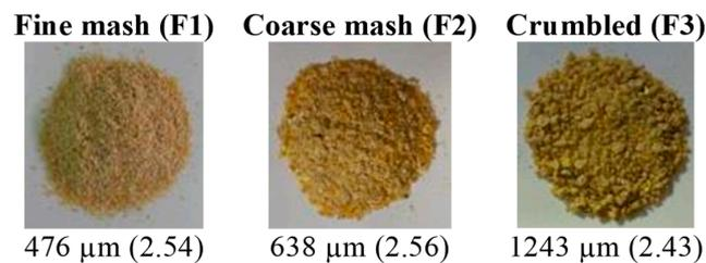
**Figure 2.** Images of the feed types used in the experiment with their respective geometric mean diameter and geometric standard deviation (between parentheses) [11].
