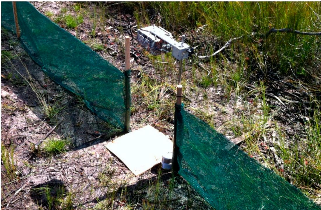
**Figure 1.** The camera overhead augmented temperature (COAT) camera-trapping method described by Welbourne [4] positions the camera-trap above a focal area that squamates are directed to by drift fences. The cork tile within the detection zone augments the thermal environment and provides the necessary thermal contrast between the target species and the background to generate detections of ectothermic species.
