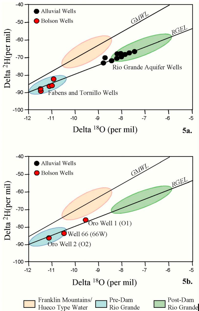
**Figure 5.** Rio Grande Aquifer samples plot in the post-dam Rio Grande region primarily while deeper bolson wells at the Cities of Fabens and Tornillo plot in the pre-dam Rio Grande range (a). Post-audit groundwater sampling for the purposes of hypothesis evaluation confirms additional well control (Well 66 and Oro Well 2) contains pre-dam water while a shallower well (Oro Well 1) near Oro Well 2 contains a mixture of pre-dam and post-dam Rio Grande water (b).
