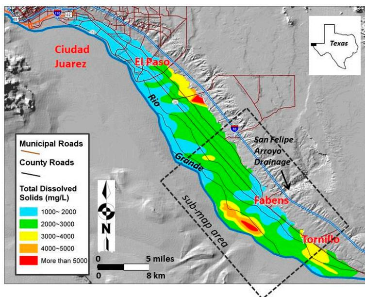
**Figure 2.** Salinity of the Rio Grande Aquifer in El Paso County, Texas. Alluvial aquifer salinities mapped by Alvarez and Buckner, 1980 using dense well control. The dilute groundwater near San Felipe Arroyo was thought to have formed by slope front recharge from the arroyo. Only the part of the Rio Grande floodplain in the United Section was mapped by Alvarez and Buckner [12]. The Rio Grande marks the southwestern limit of the section of the floodplain in the United States.
