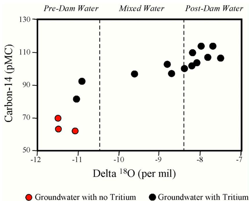
**Figure 6.** Water isotope and carbon-14 scatter plot using data from Table 2. A clear relationship is observed between isotopically light and older groundwater defined by carbon-14. Stippled vertical lines define dominant water types in the data set.
