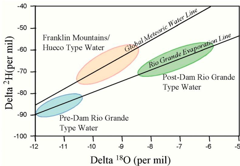
**Figure 4.** Major regional water types in the Hueco Bolson and stable water isotopes plotted for alluvial and bolson water wells sampled in this study. Regional water types include local recharge waters that characterize the Franklin Mountains/Hueco-type water and pre-dam and post-dam Rio Grande water.
