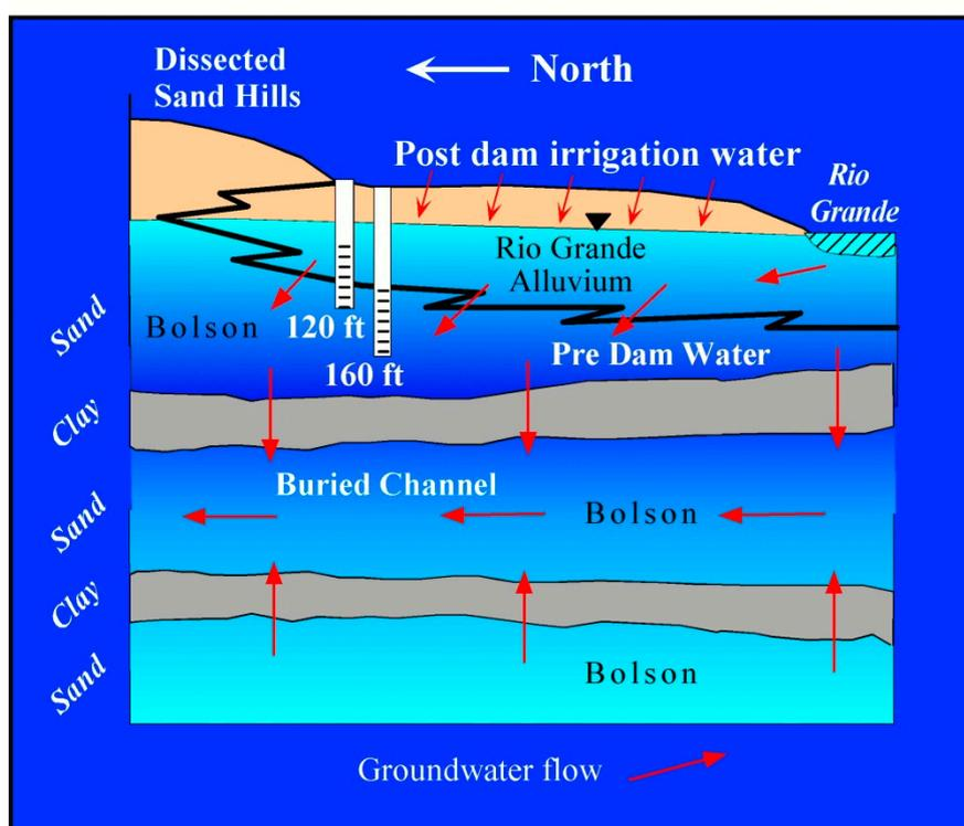
**Figure 7.** Conceptual model for groundwater flow to a deeper buried channel in the study area. The diagram frames isotope data and hydrogeologic setting at Oro Well 1 (120 ft deep) and Oro Well 2 (160 ft) in the conceptual framework image.
