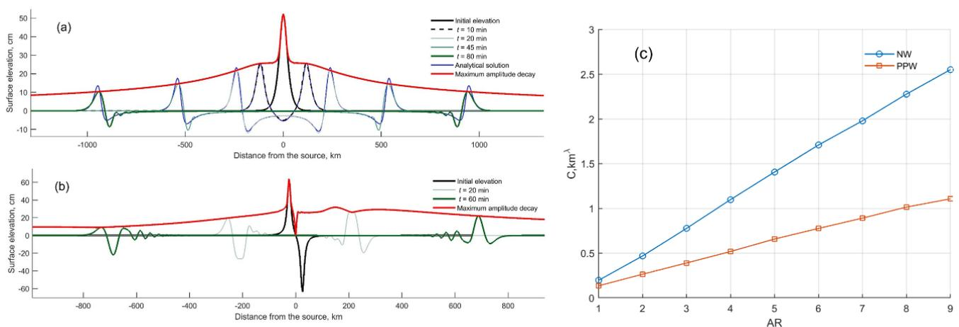
**Figure 2.** Wave dynamics with time along the centerline of the deformation in the  $x$ -direction (AR =5) from the PPW (a) and NW (b) and dependence of  $C$  on AR of the source (c).
