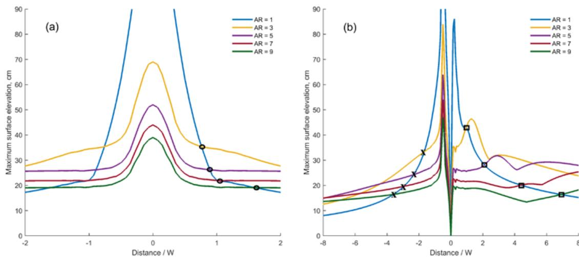
**Figure 3.** Not normalized maximum amplitudes distribution from the PPW (a) and NW (b) along the centerline of the deformation in the  $x$ -direction for the sources of different AR over constant depth. Symbols on the figure show the distance where the amplitude of the  $AR = 1$  wave decays below that of each other case.
