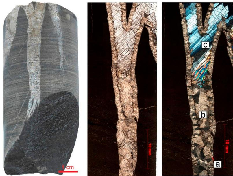
**Figure 10.** Extension fracture in limestone. Sample photo—left. Three stage of fracture filling: with calcite (a,b) and anhydrite (c). Photo of the thin section in plane-polarized light—middle and crossed polars—right. Sample depth 333.23 m (8th unit).
