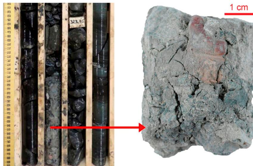
**Figure 11.** Clay-carbonate tectonic breccia at the upper boundary of the black shale units. Core photo—left. Sample photo—right. Sample depth 323.89 m (8th unit).
