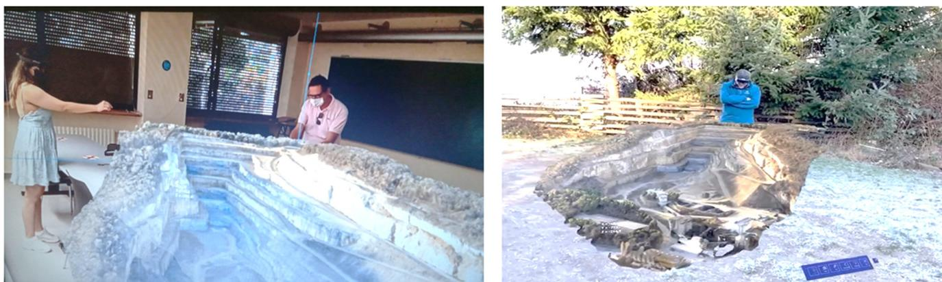
**Figure 9.** An open pit mine 3D hologram in MR. (Left) sharing the model in the classroom at the university. (Right) the model opened in the field for inspection and direct comparison with the real environment (pictures courtesy of UPC and BGC).
