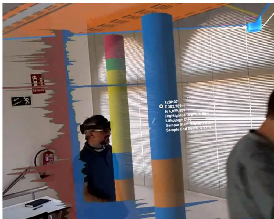
**Figure 10.** MR underground visualization (as seen in the office through the HoloLens HMD) of two boreholes (center and right) and a CPT profile (left). Pointing to the borehole, the properties of the sample are obtained at the given depth. The ground surface can be appreciated at the top (picture courtesy of BGC/Cirio).
