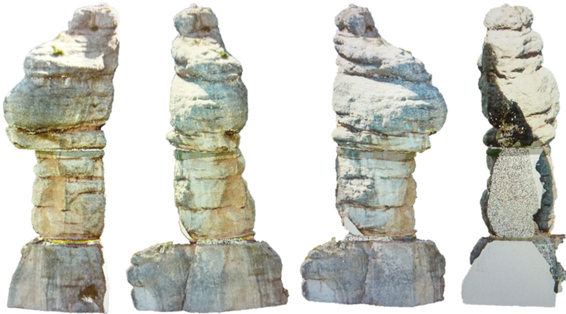
**Figure 20.** Montserrat: West, North, East and South 2D views of the “Cadireta” 3D model, prior to the FEM mesh generation. Note in the picture on the right (partially hidden side) the planes added to the surface of the base of the column to close the volume.
