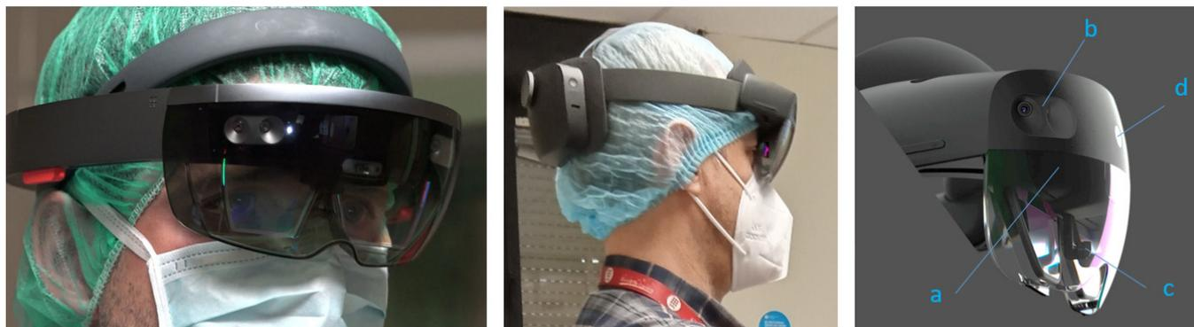
**Figure 3.** Microsoft’s HoloLens MR see-through holographic HMD. (Left) HoloLens 1. (Center) HoloLens 2. (Right) detail of some built-in sensors: (a) MEMS projector; (b) two visible-light cameras for head tracking; (c) IR camera for eye tracking; (d) depth sensor.
